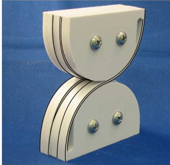
Figure 1.5: A compliant rolling-contact element.
