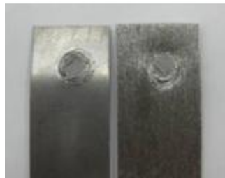
Figure 7 Fracture in weld
