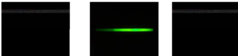
Figure 5.3. Low adsorption of proteins on a PEG monolith. (A) Background; (B) After loading with FITC-BSA; (C) After flushing with aqueous buffer.
