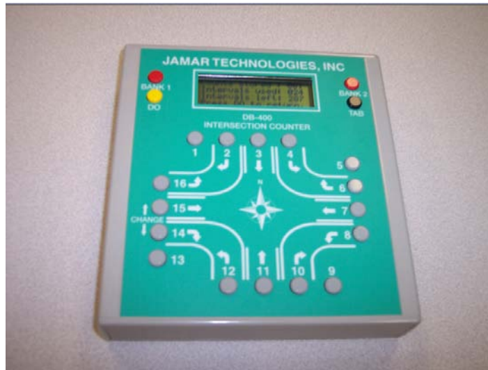
Figure 3-9: The electronic counter used
