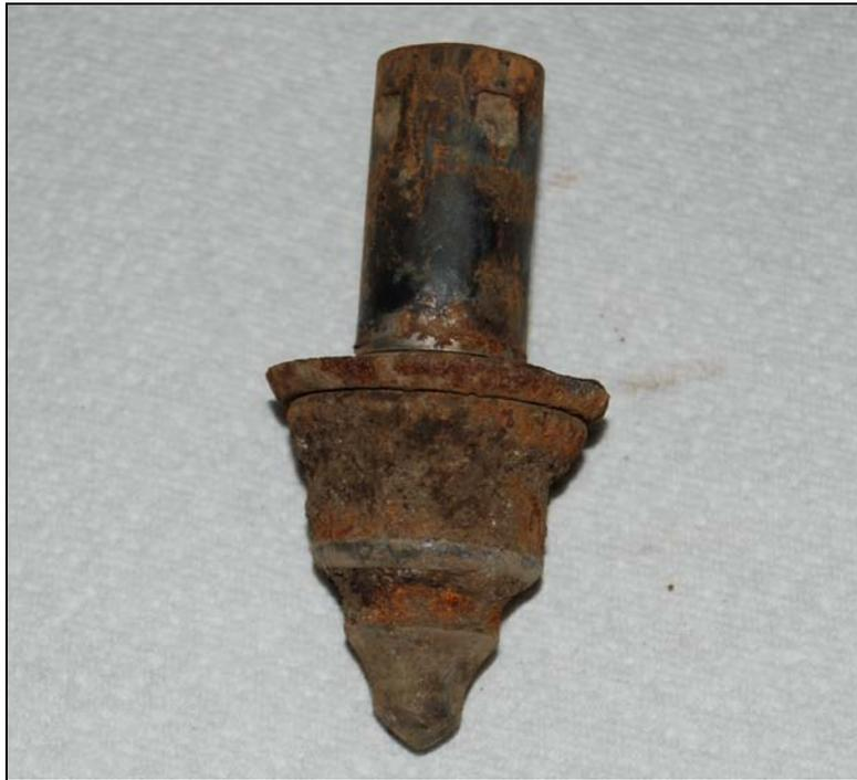
**Figure 3.1 Picture of gouge tooth used during testing**
