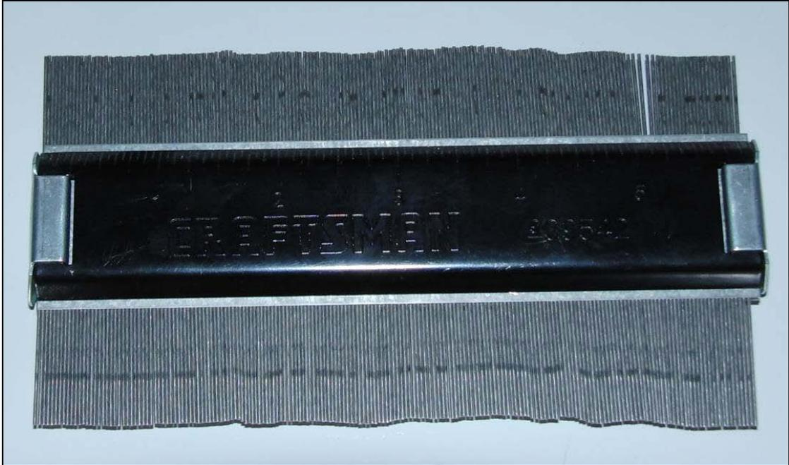
Figure 3.4 Contour gage used for profile measurements
