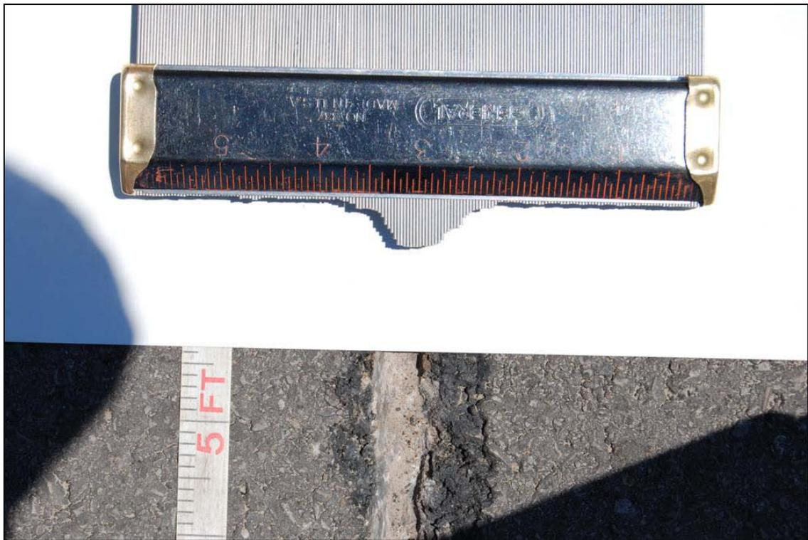
Figure 3.5 Example of photograph used to record gouge profile
