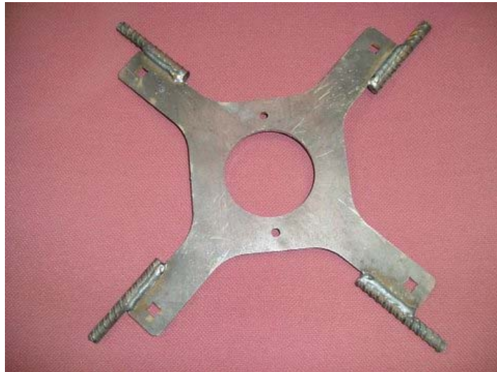
Figure 4-6 Metal Star used in Gauge Installation and Assembly for Salt Lake City, UT
