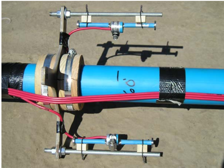
Figure 4-7 Completed Assembly of Star and Gauges Attached to Inclinator Pipe for Installation
