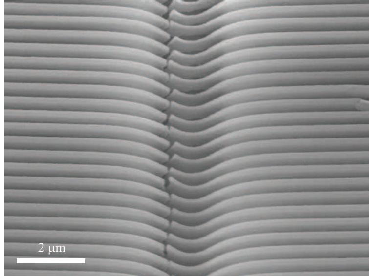
Figure 10.13: SEM image of ZEP gratings written in the core of an optical fiber. Note that the grating contrast is so high that the bottom of the grating is not visible from this view.
