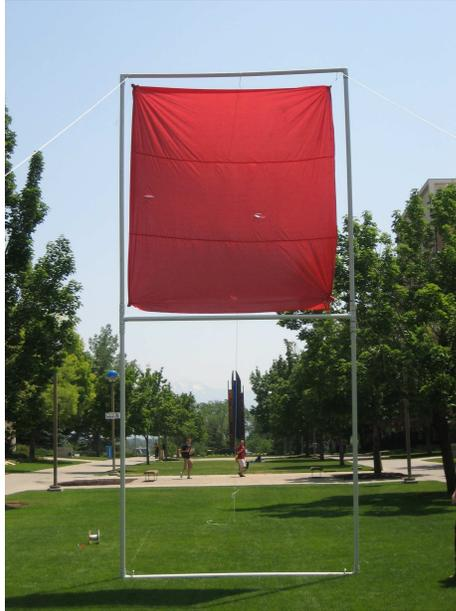
**Figure 3.20:** The obstacle is an elevated red banner. Color segmentation finds the obstacle in the image plane.
