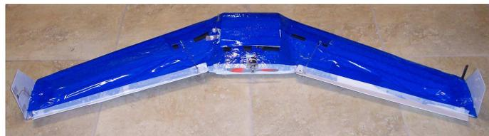
**Figure 3.21:** The MAV has a wing span of approximately 48 inches and uses the Kestrel autopilot.
