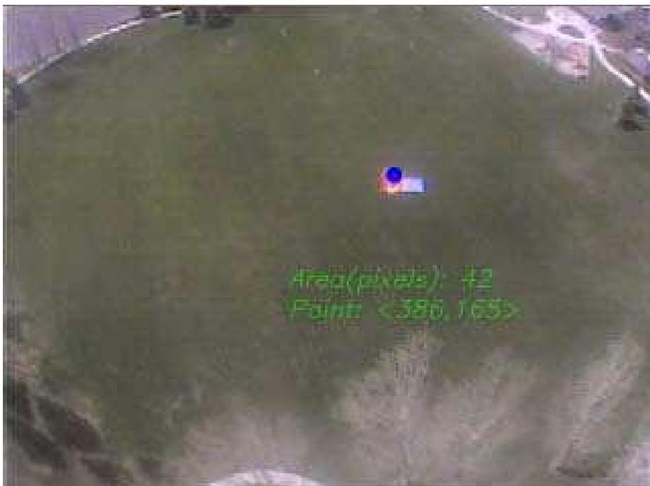
**Figure 4.17:** The ground station processes video by color segmentation to find the location of the red cloth.
