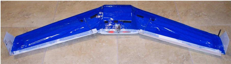
**Figure 4.15:** The MAV has a wing span of approximately 48 inches and uses the Kestrel autopilot from Procerus Technologies.
