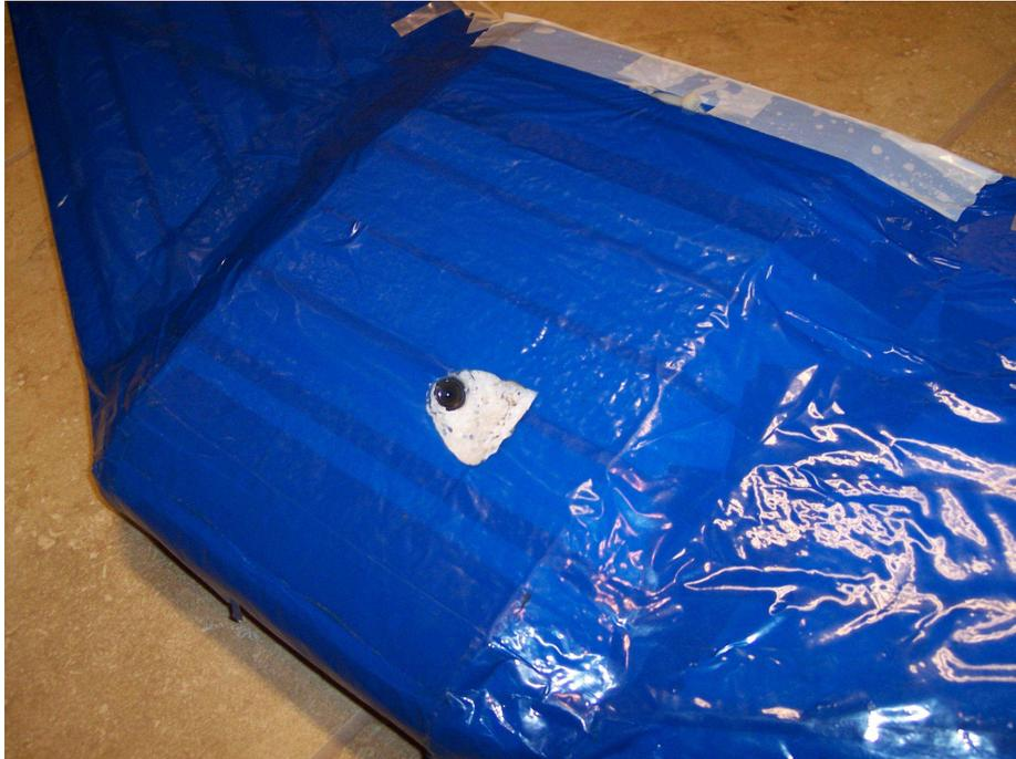
**Figure 4.16:** The camera is mounted under the MAV at an elevation angle of  $30^\circ$ .
