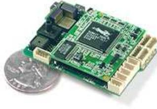
**Figure A.2:** The Procerus autopilot is used for hardware-in-the-loop simulations.
