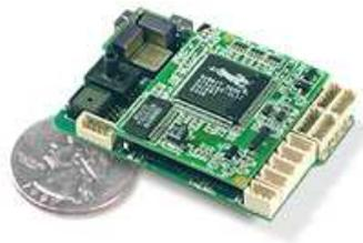
**Figure 3.22:** The Kestrel autopilot onboard the MAV is compared to the size of a quarter.
