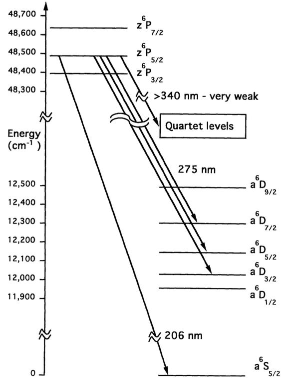
FIG. 2.—Partial Grotian diagram showing the decay of the  $z^6P^{\circ}_{5/2}$  level of Cr II with approximate vacuum wavelengths. The unspecified quartet levels to which transitions have been observed include the  $a^6D_{3/2}$ ,  $a^6D_{5/2}$ ,  $a^6D_{7/2}$ ,  $a^4P_{5/2}$ , and  $b^4P_{3/2}$  levels (Kiehl 1951).
