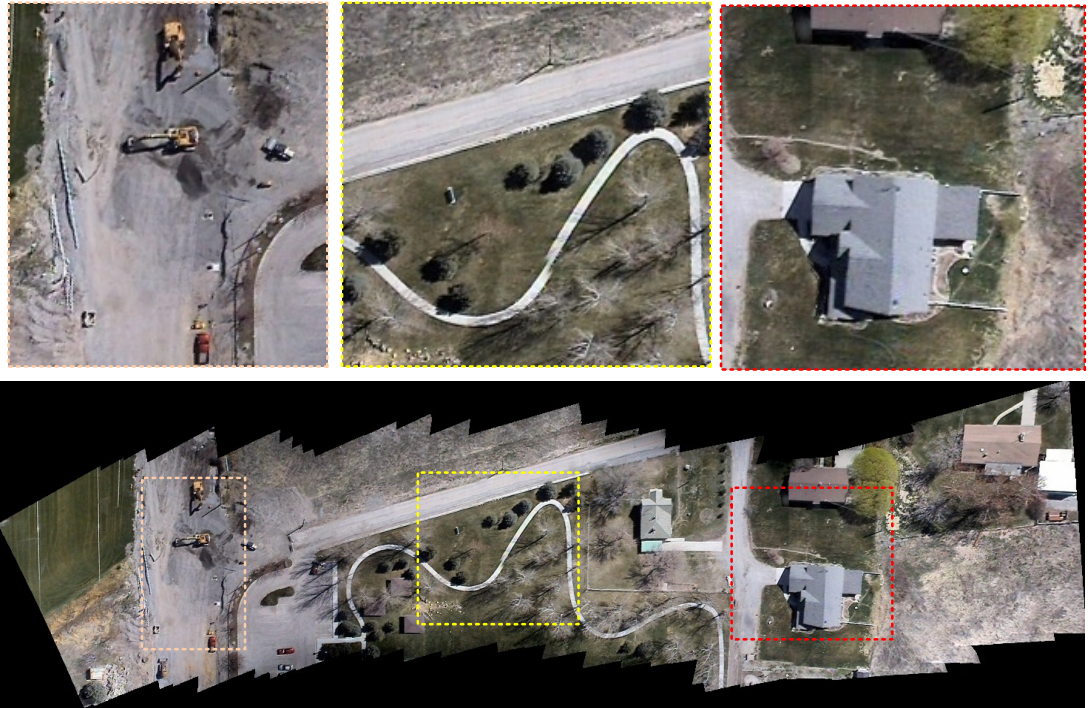
Figure 4.5: This figure shows the quality of an actual MAV mosaic created using 600 MAV images of Vineyard in Utah.
