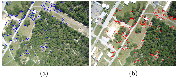
Figure 2.14: This figure shows the results of the SURF feature detector when applied to two MAV images.
