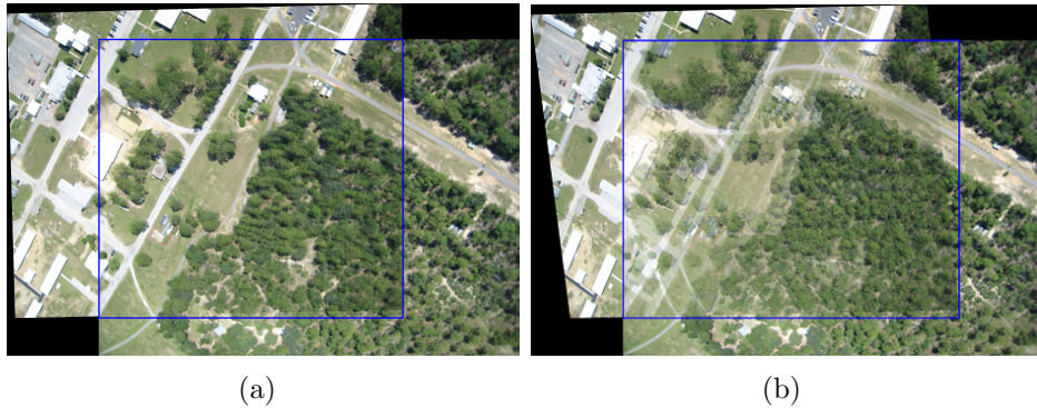
Figure 2.17: This figure shows how inaccuracies in an estimated perspective transformation affect the resulting composite image.
