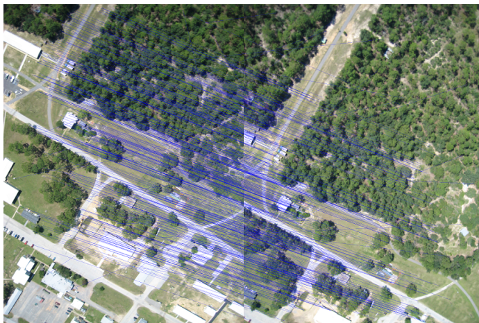
Figure 2.15: This figure shows the correlation of SURF feature detectors using the same two MAV images used in Figure 2.14. This figure has been rotated 90 degrees for display purposes.
