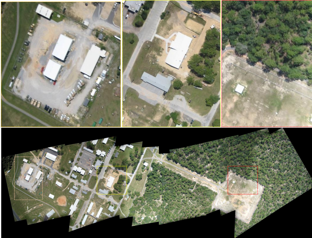
Figure 4.6: This figure shows the quality of an actual MAV mosaic created using 17 high-resolution images of Florida location.
