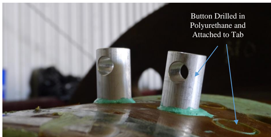
Figure 5. Pull Tabs Attached to the Polyurethane Clamp in Preparation for the Button Pull Test.
