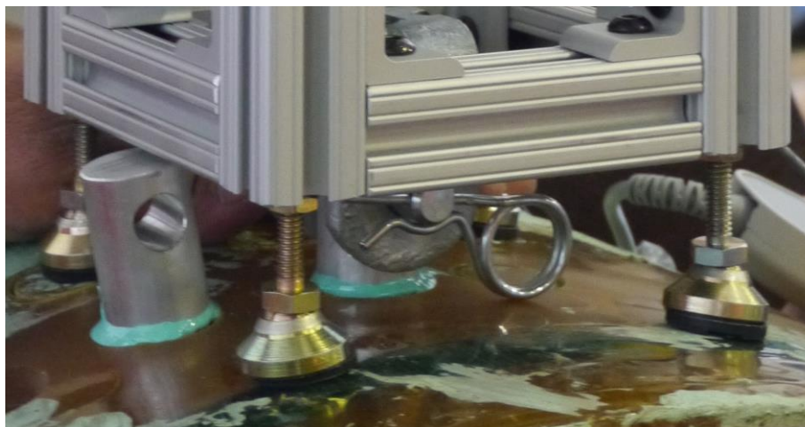
Figure 6. Device to Measure Tensile Strength of the Adhesive Clamp by Pulling the Button Tab to Failure.
