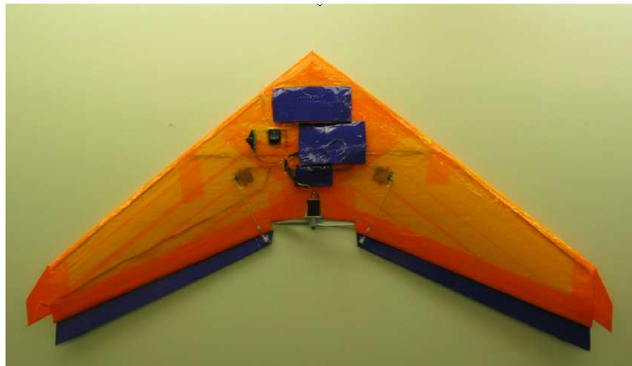
Figure 2.5: The Flight Test MAV. The MAV used in the flight testing of the attitude estimation and aerobatic maneuvering control laws.
