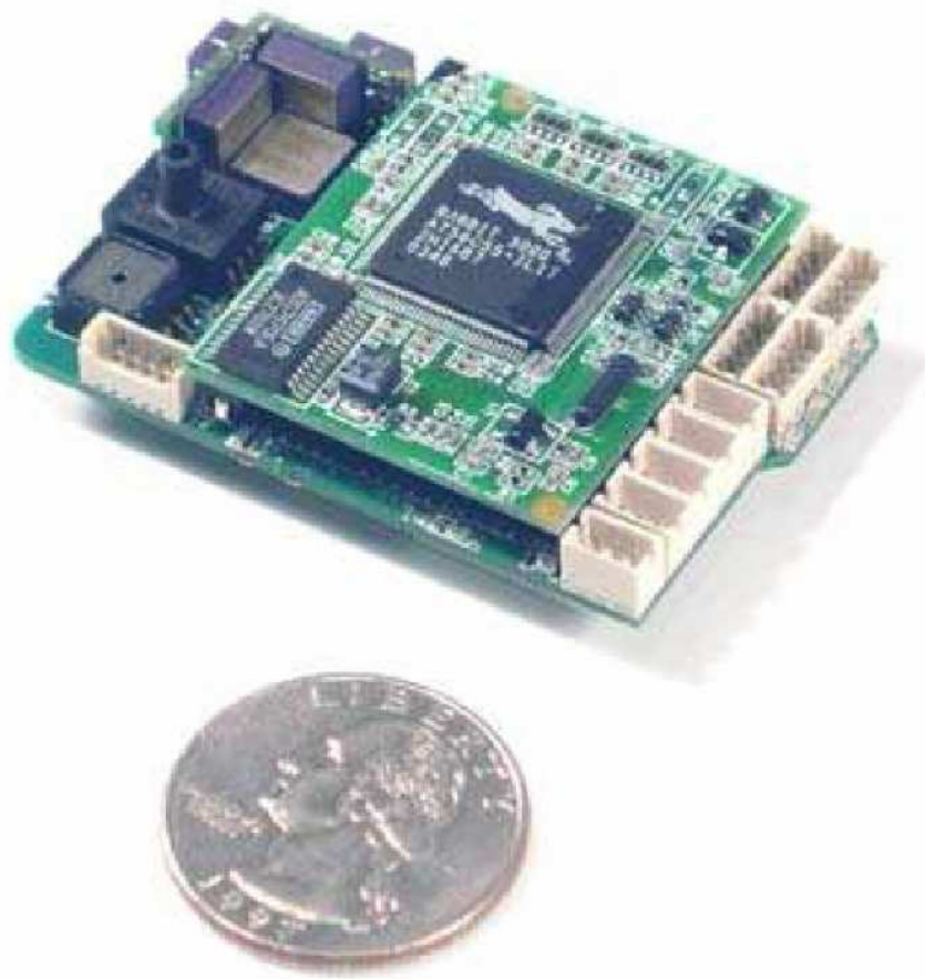
Figure 2.6: The Kestrel Autopilot. Version 2.2 of the autopilot is shown with a quarter for scale purposes.
