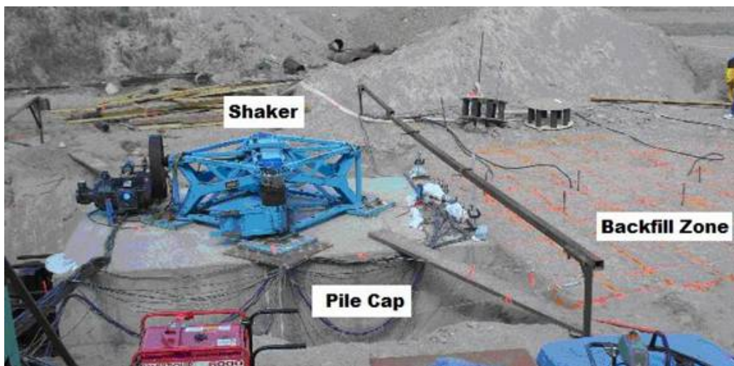
Figure 3.5 Photos of test site and equipment setup
