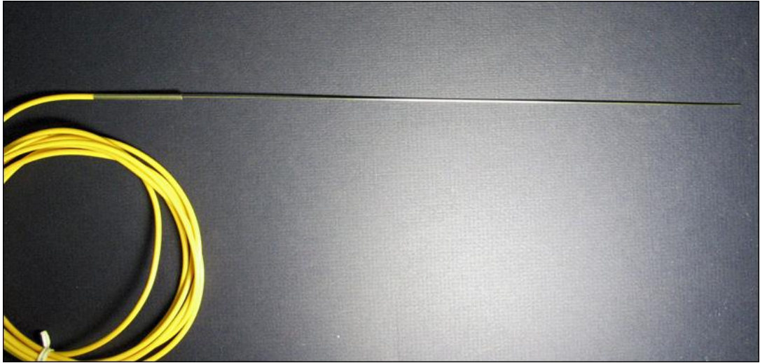
Figure 5.14: One of the SR-FBG high temperature probes installed into the test aircraft.
