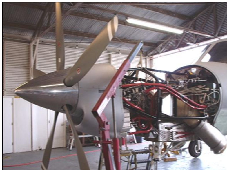
Figure 5.13: The engine compartment of the aircraft where the SR-FBG high temperature probes were installed.
