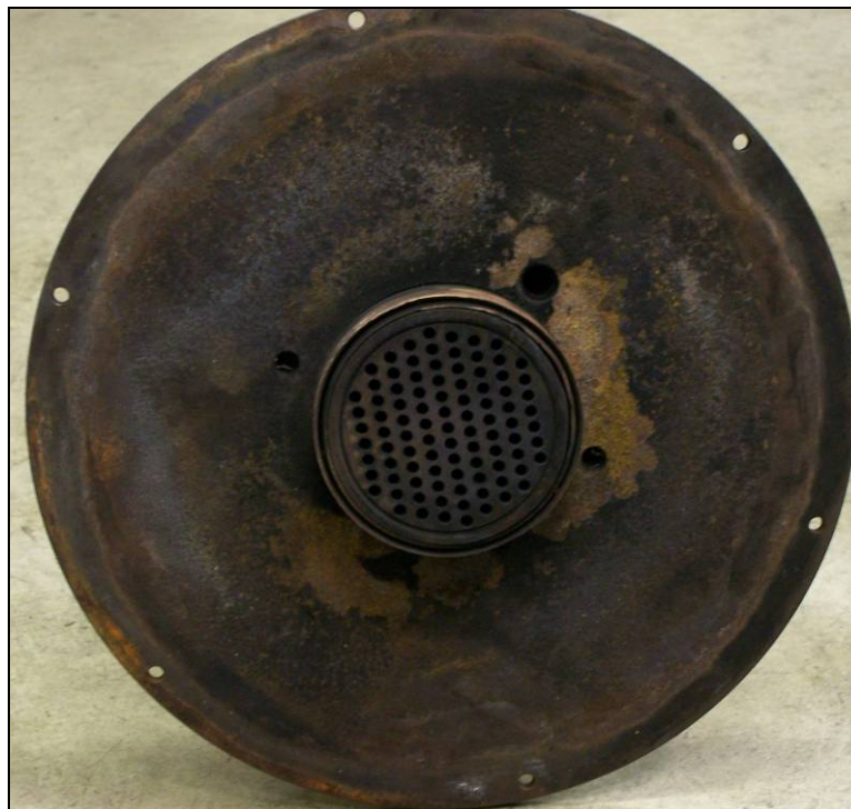
Figure 30. The burner face and top flange of the MFR. The cast refractory material fits closely around the burner face. The fact that this water-cooled assembly rests directly on top of the first reactor section is one reason for lower wall temperatures at the top of the reactor.
