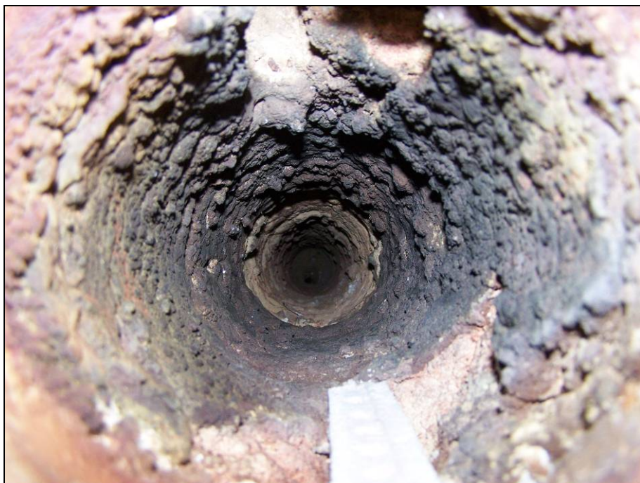
Figure 32. Looking down into the MFR with the burner removed reveals ash deposits with colors characteristic of the oxidizing and reducing conditions in different regions of the MFR.
