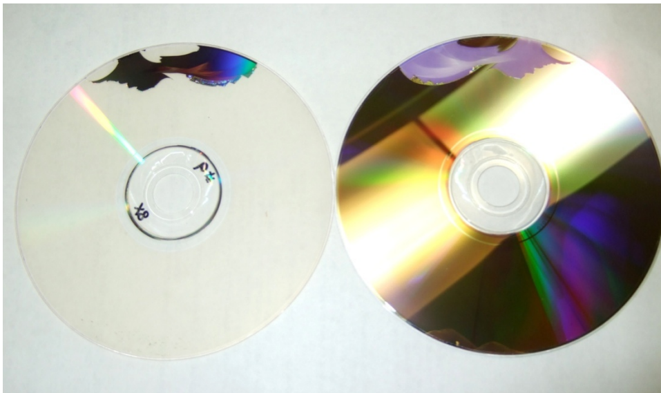
Figure 4.8 – Dummy substrate (left) separated from disc (right).
