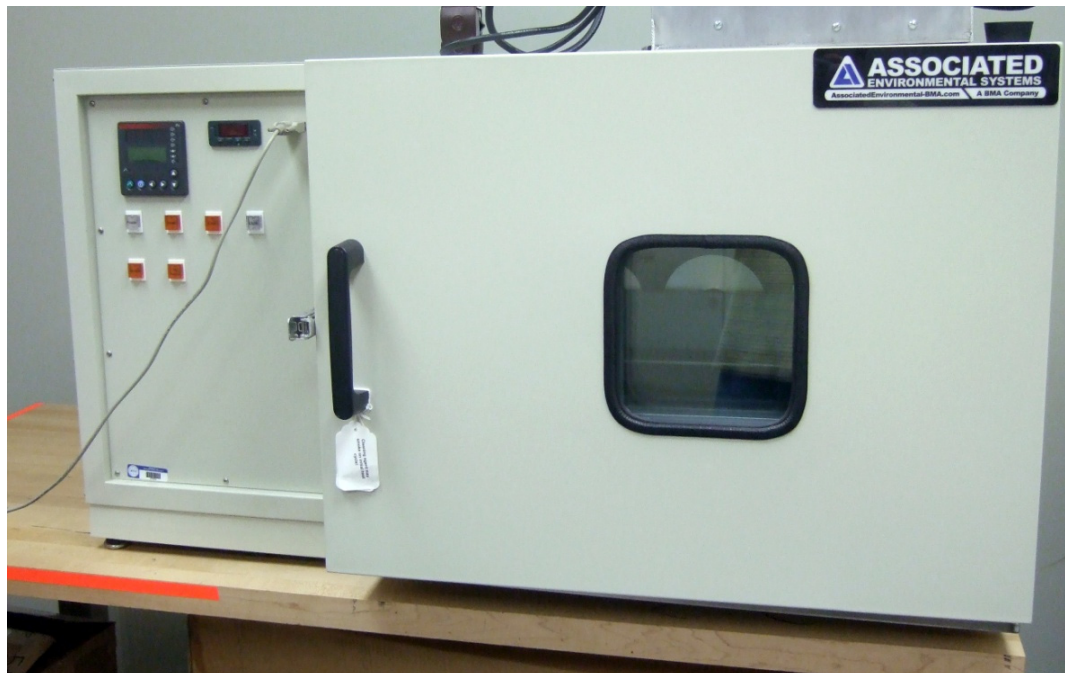
Figure 3.2 – BHD-203 test chamber from Associated Environmental Systems
