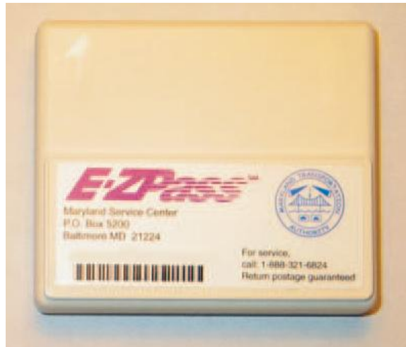
Figure 2.2: An active RFID tag used in collection of highway tolls [2].
