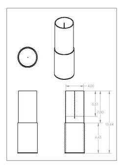
Figure 3F - Convex Angular Flow Test Fixture
