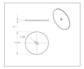
Figure 3C - Concave Angular Flow Bottom Plate 0.38 Inch Hole
