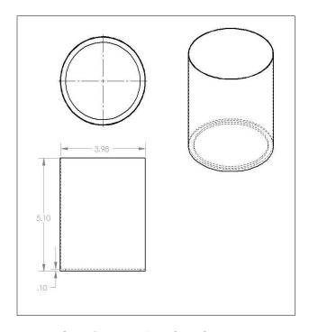
Figure 3B - Concave Angular Flow Test Fixture
