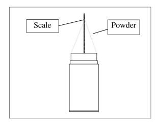
Figure 31 - Convex Angular Flow Test Fixture: Down Position
