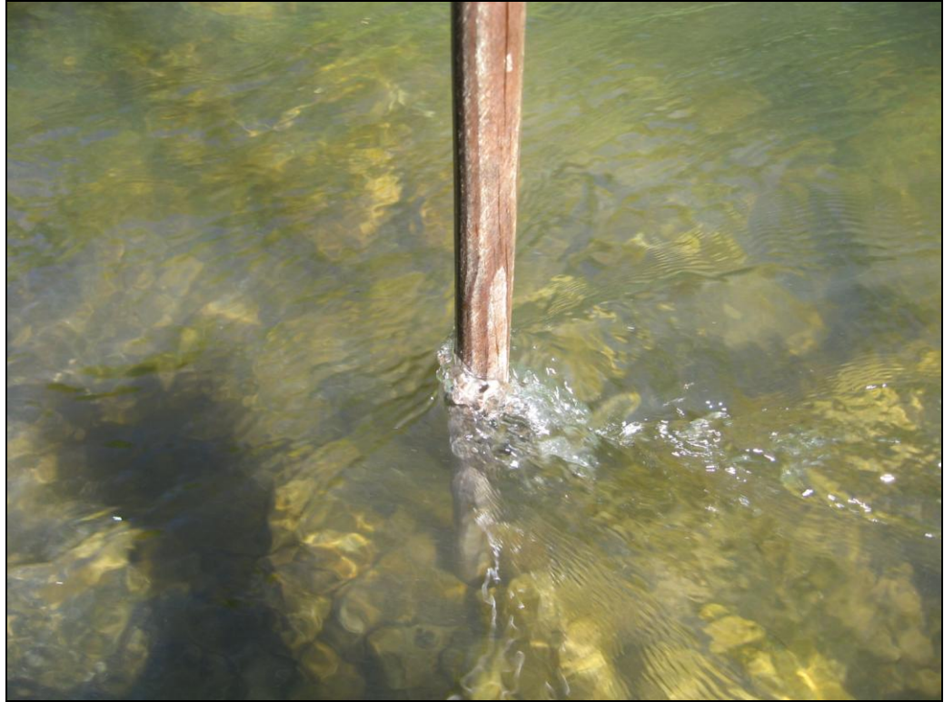
Figure 4-7: Critical Flow Wave Action on Wading Staff
