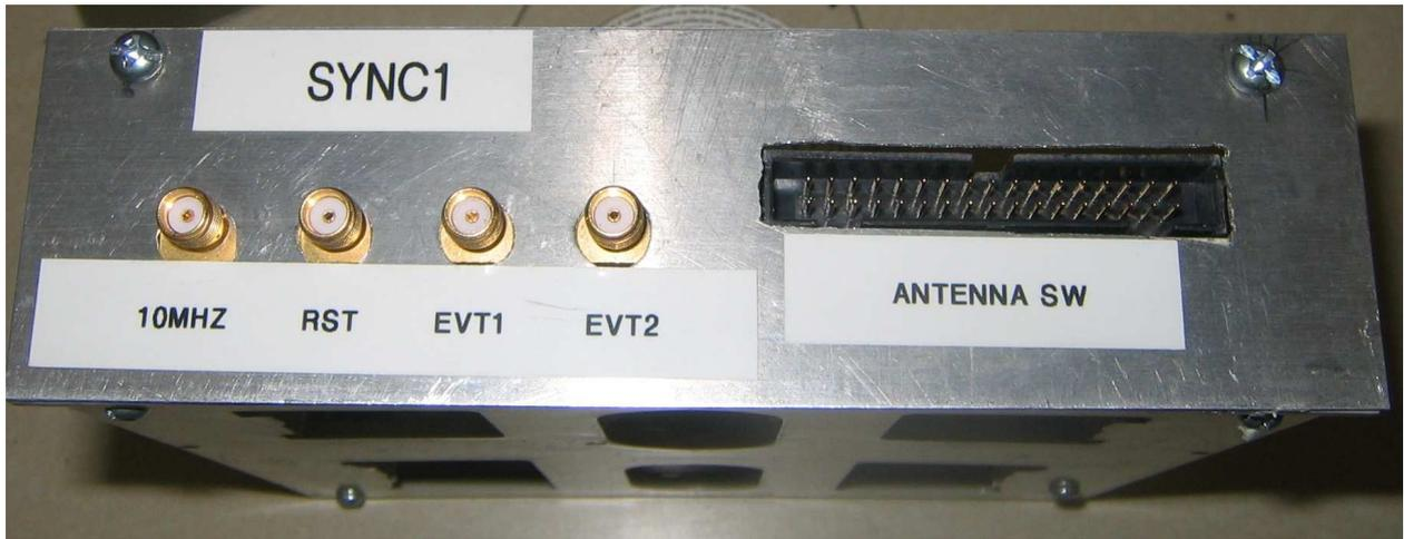
Figure 3.8: Front panel of the SYNC module with inputs for 10 MHz clock and reset, and outputs for events and antenna control
