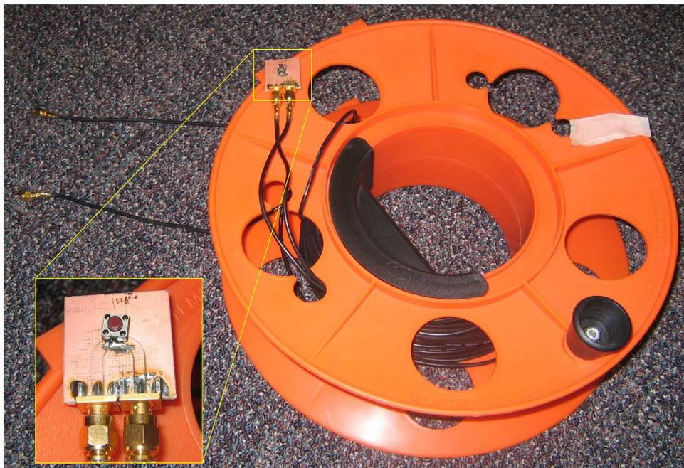
Figure 3.5: Trigger connected to two transmission lines, allowing simultaneous reset of two SYNC boards
