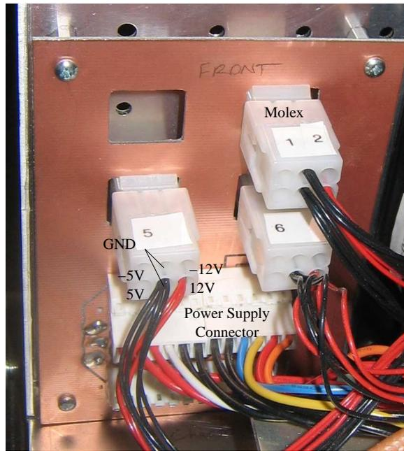
Figure 3.17: power card used to connect the power amplifiers
