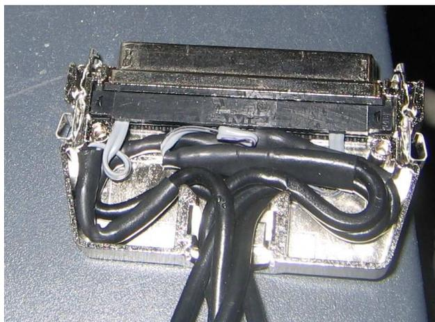
Figure 3.24: Photo showing connections for NI adapter cable
