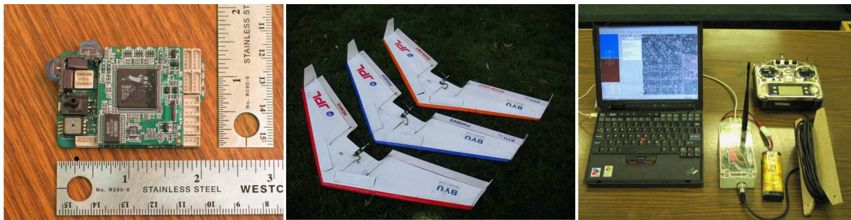
Fig. 13. Hardware platform used to obtain experimental results. The first frame shows the Kestrel autopilot designed at BYU. The second frame shows the airframes used for this study. The third frame shows the ground station components for our testbed.
