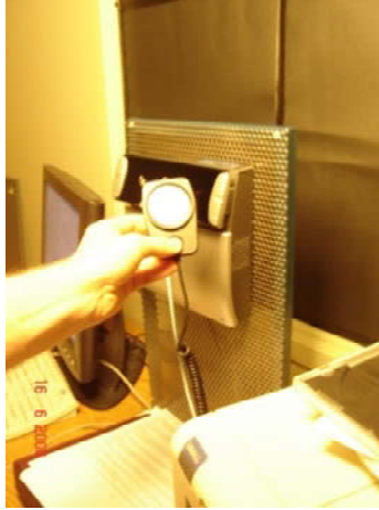
Figure 3-4 Davis Instrumentations Photometer
