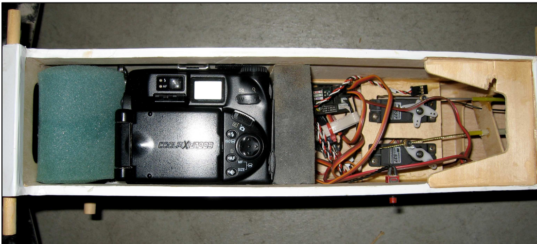
The camera inside the aircraft.. The DigiSnap was located under the nose hatch and the Gecko was secured on top of the nose hatch by Velcro and a rubber band.
