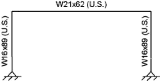
Figure D-1 Special moment frame members (Richards and Prinz, 2007)
