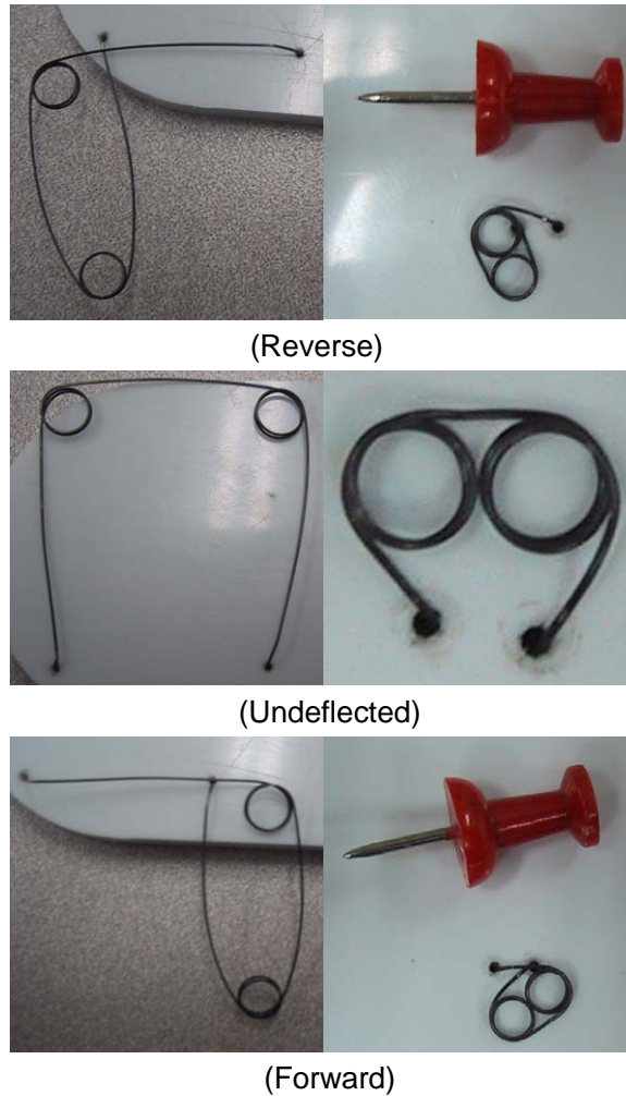
Figure 4.6: Photographs of two different tristable compliant mechanisms with torsional springs.
