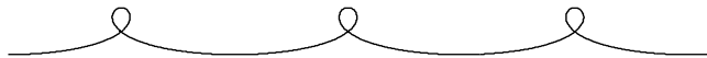
Figure 5.1: For a UAV orbiting a moving target, the trajectory exhibits loops corresponding to the times when the UAV and the target are moving in opposite directions and long arcs when both are moving in the same direction.
