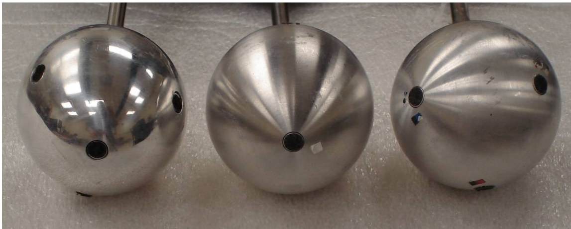
Figure 2–9: From left to right orthogonal, tetrahedron and six-microphone AED probes
