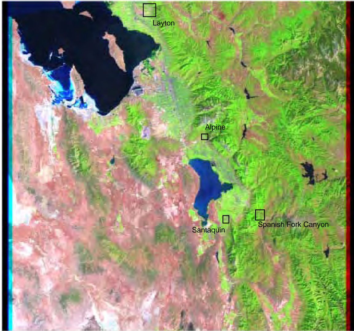
Figure 2: The study areas for this research - Landsat 7 scene, path 38, row 32, May 28, 2000. The image is displayed as 7, 4, 2; middle infrared (band 7) in the red plane, near infrared (band 4) in the green plane and green (band 2) in the blue plane. The four study areas are marked.
