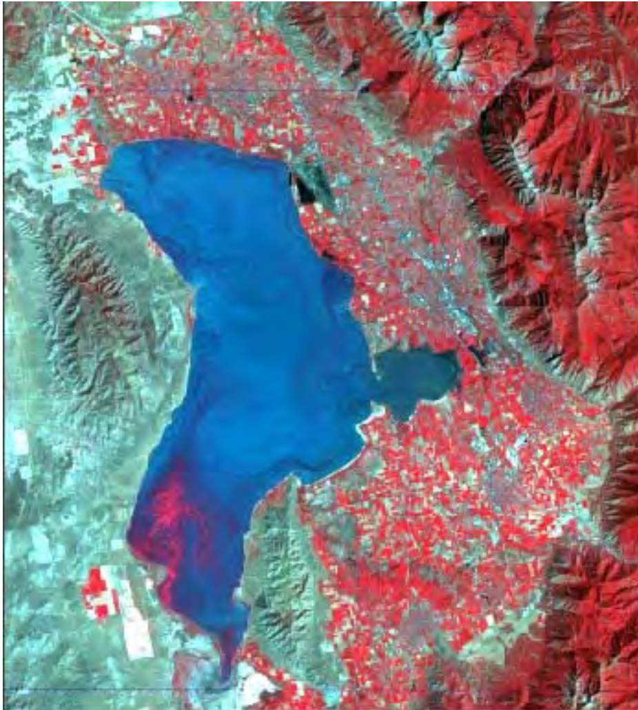
Figure 1: Landsat-7 ETM+ subset image of Utah Valley, May 28, 2000. Near infrared (band 4) shown in the red plane, red (band 3) shown in the green plane and green (band 2) shown in the blue plane.
