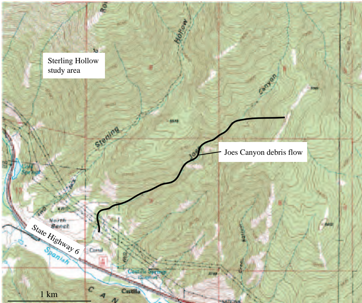
Figure 14: Topographic map of Sterling Hollow and Joes Canyon, and path of Joes Canyon debris flow.
