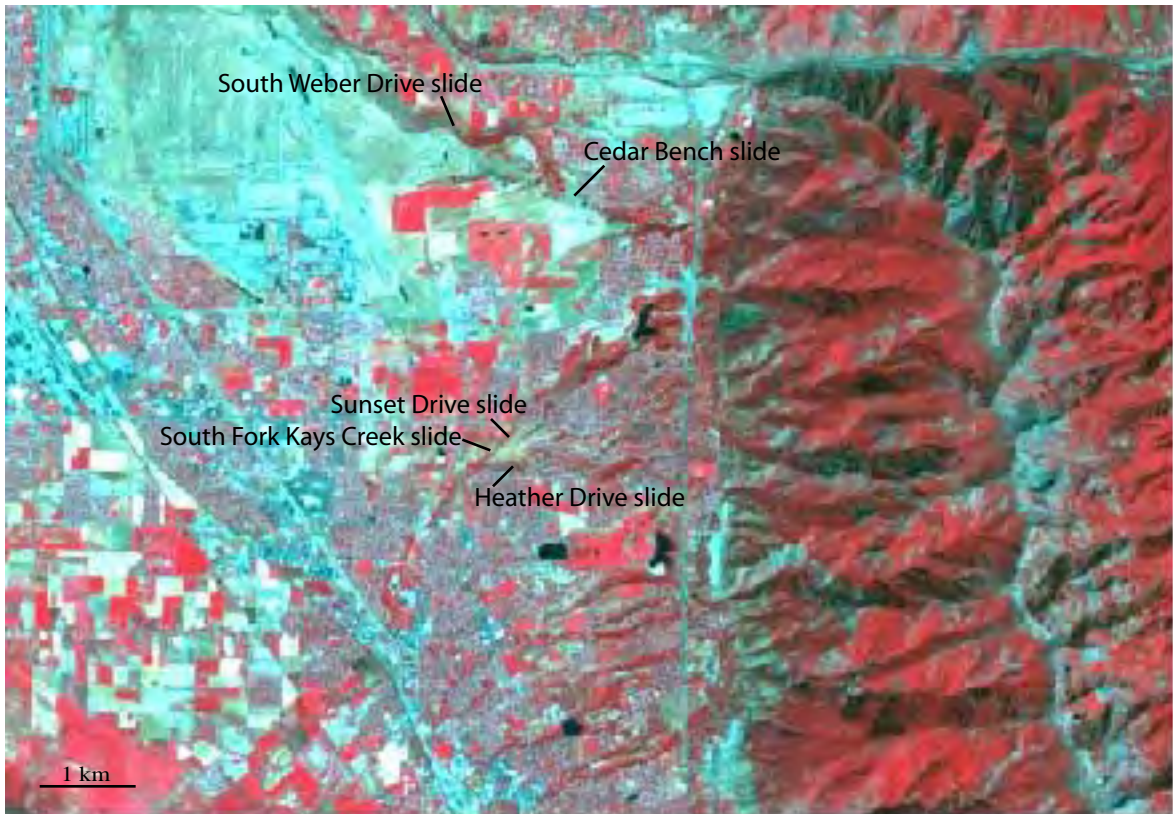
Figure 3: Landslides (1998-2001) of the Layton and South Weber area. The image was taken on May 28, 2000 and is displayed as bands 4, 3, 2.
