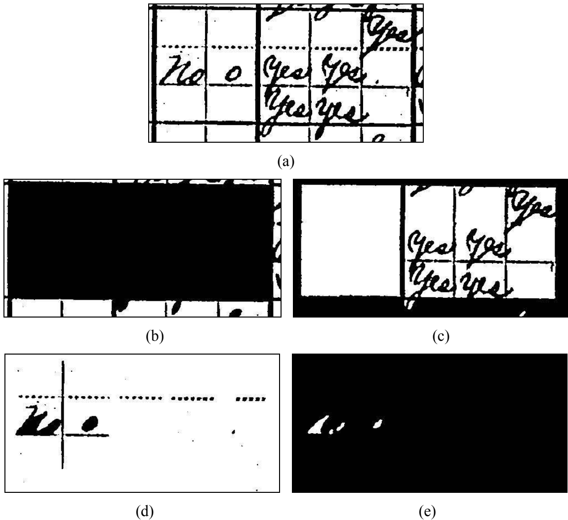
Figure 3.3 Contour Layers for Sample Image. (a) Original Image (b) First “Black” Layer (c) Second “White” Layer (d) Third “Black” Layer (e) Fourth “White” Layer
