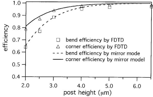
Fig. 5. Efficiency as a function of post height.
