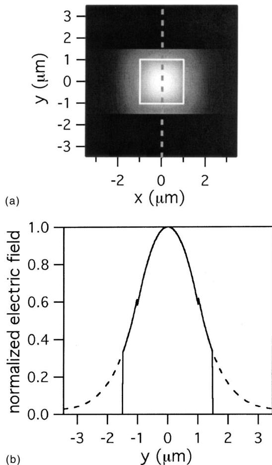
Fig. 6. Clipping of a mode by a perfect mirror. (a) Mode clipped by a perfect mirror  $3\ \mu\text{m}$  tall in the  $y$  dimension. (b) Clipped field profile along the dotted line in (a). Dashed curve, clipped part of the mode.
