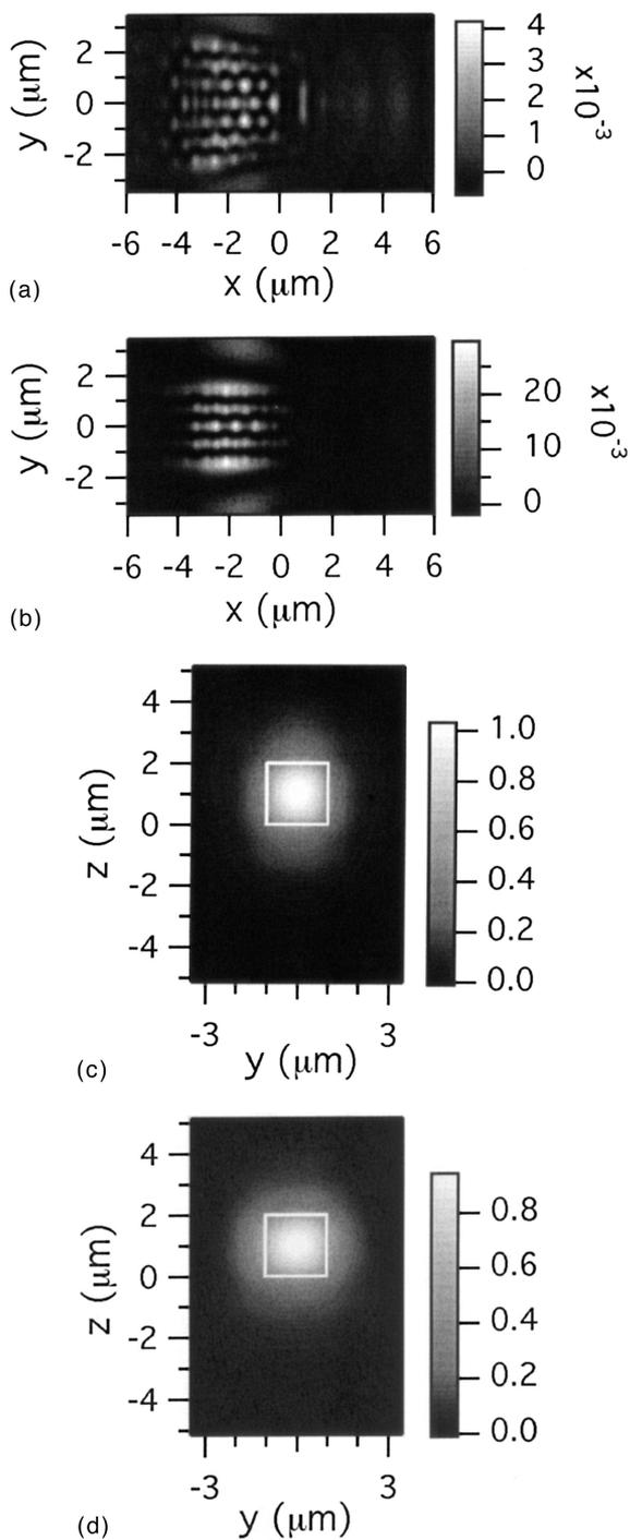
Fig. 4. Case 1 (5.0- $\mu\text{m}$  post height), case 2 (3.0- $\mu\text{m}$  post height). (a)  $z$  component of Poynting vector,  $z = 5.1 \mu\text{m}$ , case 1. (b)  $z$  component of Poynting vector,  $z = 5.1 \mu\text{m}$ , case 2. (c)  $E_y$  amplitude,  $x = 5.0 \mu\text{m}$ , case 1. (d)  $E_y$  amplitude,  $x = 5.0 \mu\text{m}$ , case 2.
