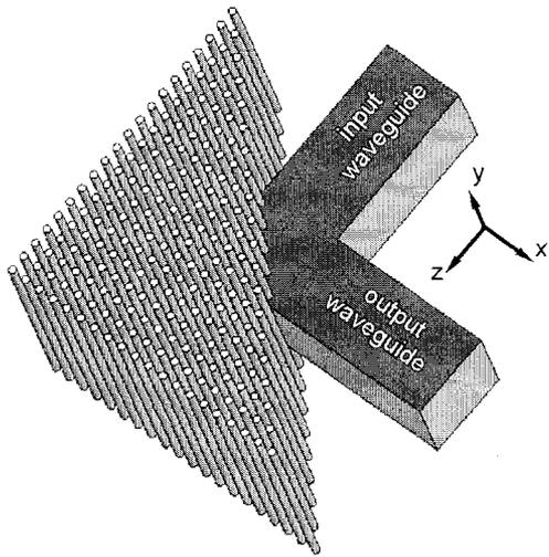
Fig. 1. Hybrid PhC-CWG 90° bend. See text for details.
