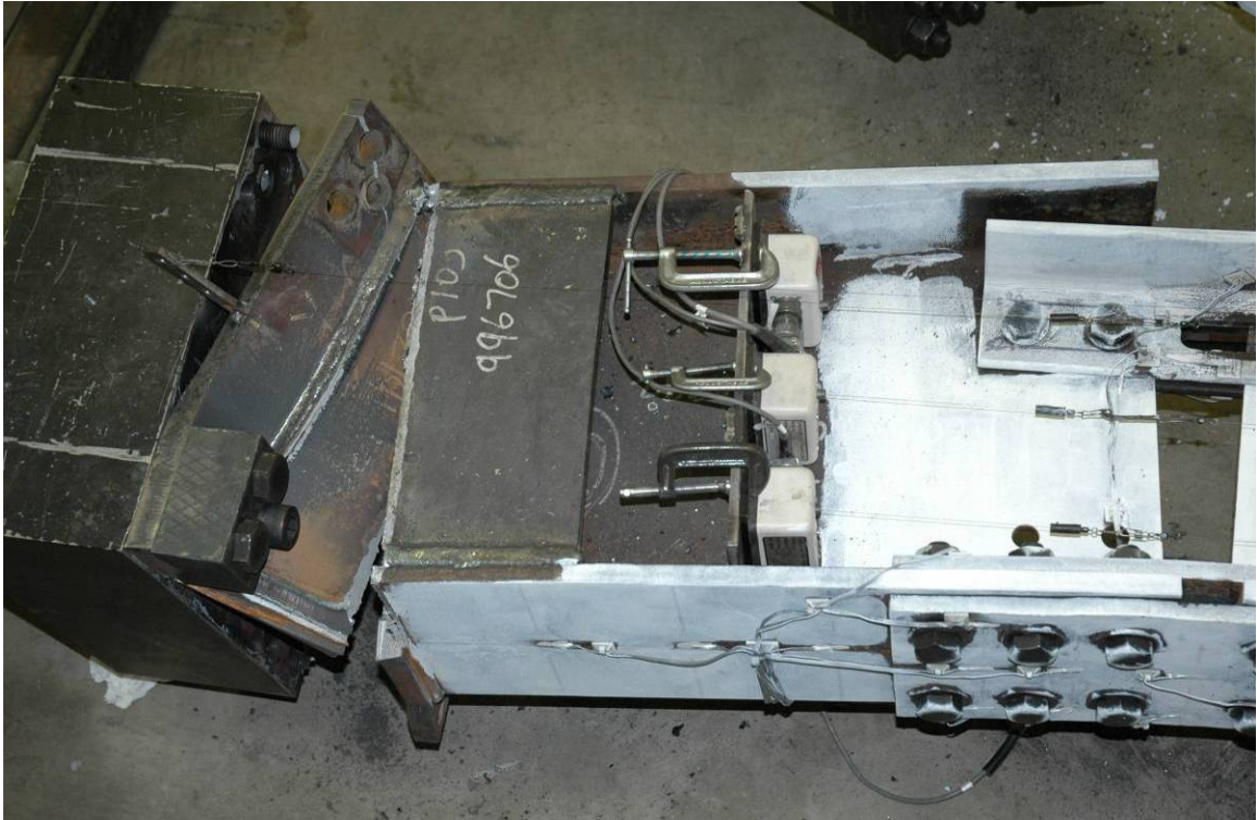
Figure 3-26 Specimen 2 – Boundary Plate Failure
