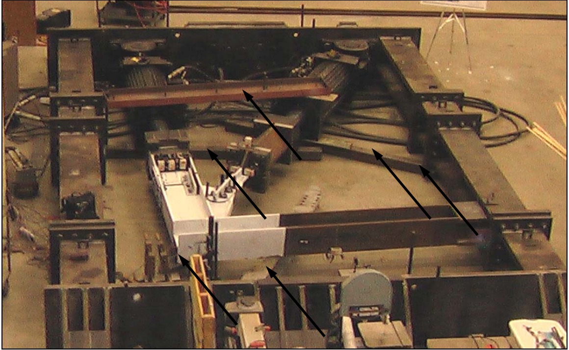
Figure 2-7 Specimen 2 – Out-of-Plane Bracing
