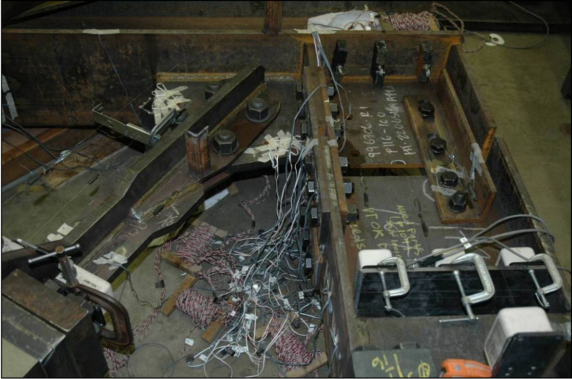
Figure 2-16 Specimen 1 – Gusset and Splice Plate Instrumentation
