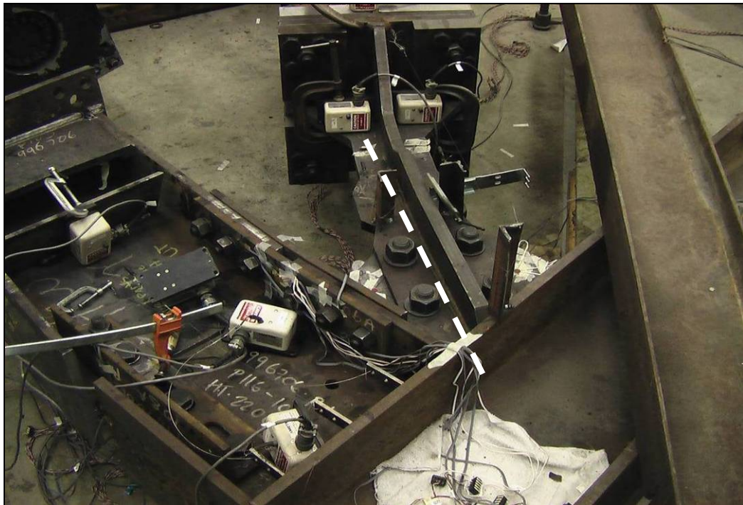
Figure 3-4 Specimen 1 – Connection Deformation Following Boundary Failure
