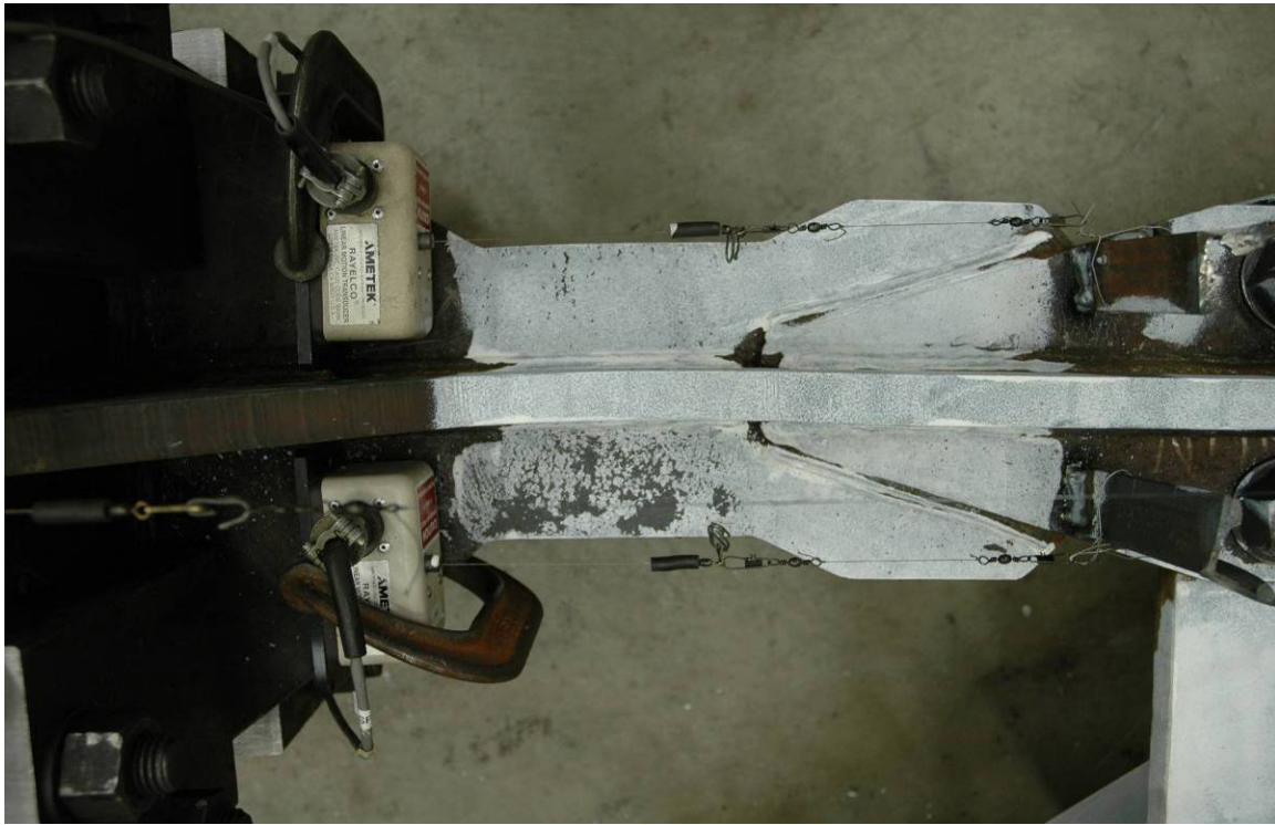
Figure 3-25 Specimen 2 –Yielding of BRB Core Extension Assembly (6.5% Drift)
