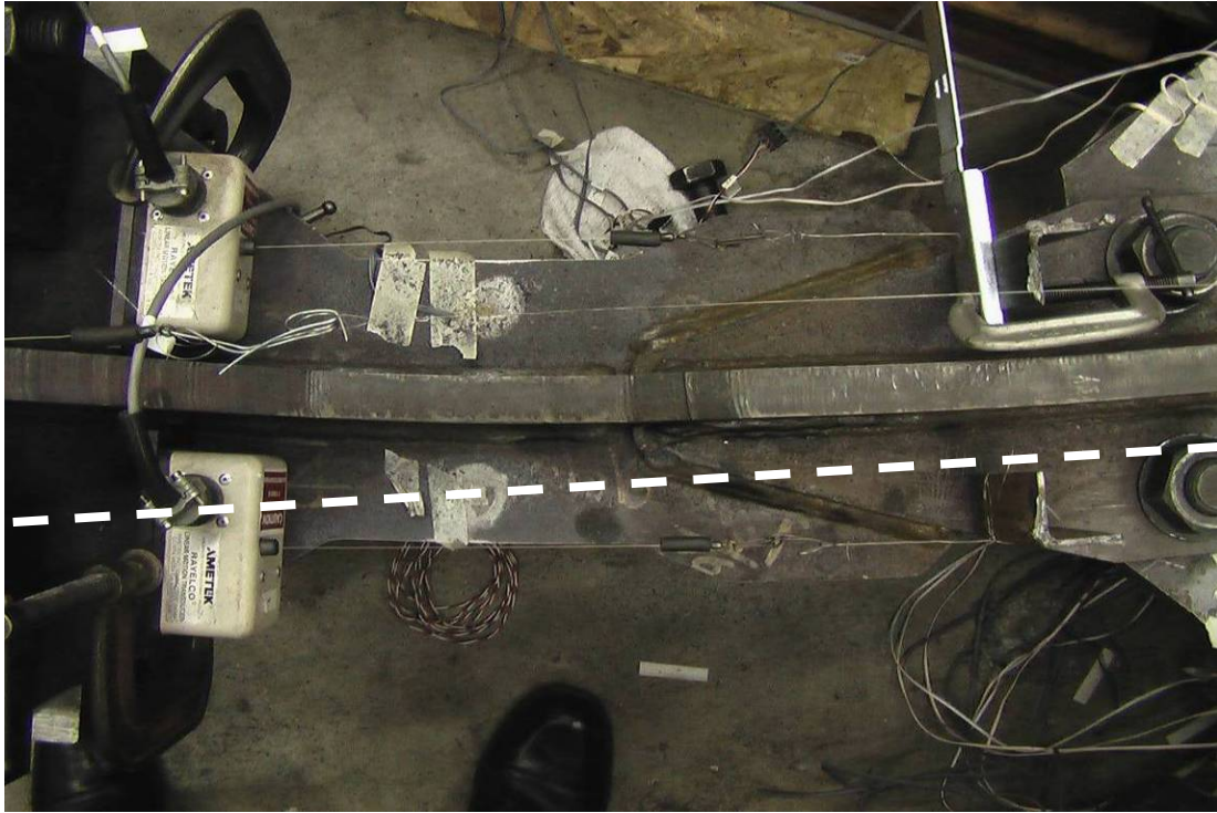
Figure 3-5 Specimen 1 – Core Extension Deformation Following Boundary Failure
