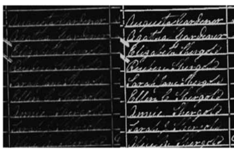
Figure 8. Selective Stroke Enhancement using a custom convolution kernel derived from the handwriting.
