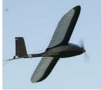
**Figure 2-16. The flexible composite airframe built by the USAF and University of Florida. [25]**
