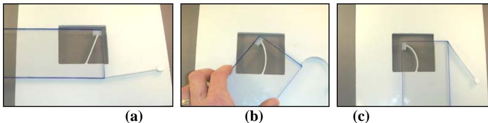
**Figure 5-6. Motion of the concept from Figure 5-5 in the (a) deployed, (b) transition, and (c) stored configurations.**
