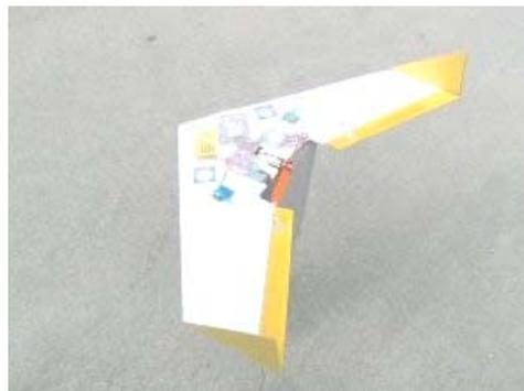
**Figure 5-17. IRIS, BYU's 45 cm wingspan 'flying wing' UAV.**
