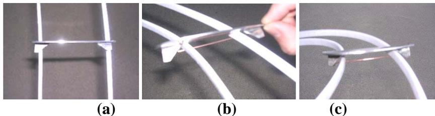
**Figure 4-23. Detailed view of the motion for the prototype shown above. (a) Top view shows the feet which keep the rib upright. (b) As the flexible segments move inward, the rib begins to fall. (c) In the final position, the rib lies flat against the supporting segments.**
