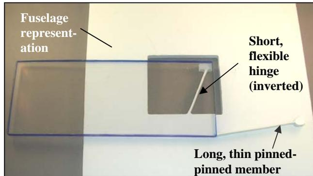
**Figure 5-5. Bistable joint concept with reduced footprint**
