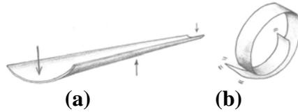
**Figure 4-10. Bi-stable arched metal strip used in slap bracelets. By deflecting the center of the strip (a), it collapses into its other (coiled) stable equilibrium position.**
