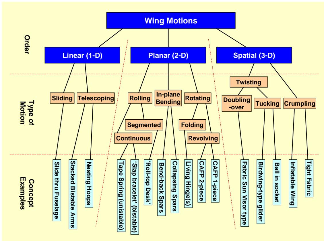
Figure 4-1. Classification System for Deployable Wing Motion Types.
