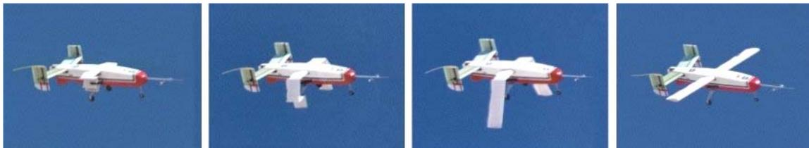
**Figure 2-20. Deployment sequence for NASA's I2000 inflatable glider.**
