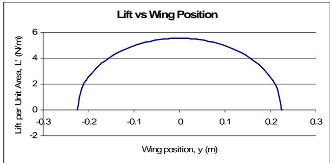
**Figure 5-20. Elliptical Lift Distribution for the BYU UAV.**
