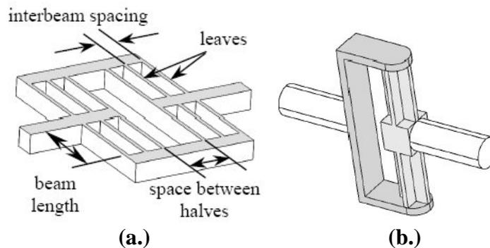
**Figure 2-26. (a) The compliant translational and (b) Compliant revolute joints. [39]**
