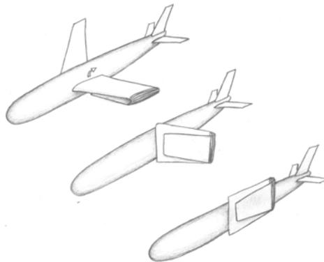
**Figure 4-21. A hybrid folding and tucking wing concept.**
