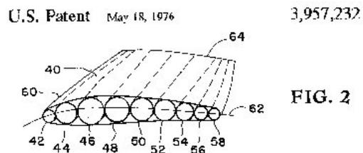
**Figure 2-18. Inflatable wing patent assigned to Wayne Sebrell, 1976. [27]**
