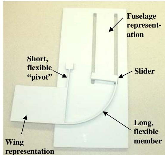
**Figure 5-3. Compliant slider-crank five-bar mechanism.**
