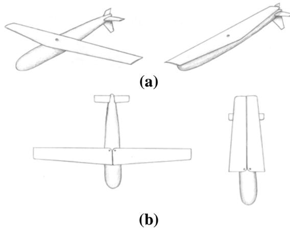
**Figure 4-15. (a) One-piece and (b) two-piece rotating wing.**
