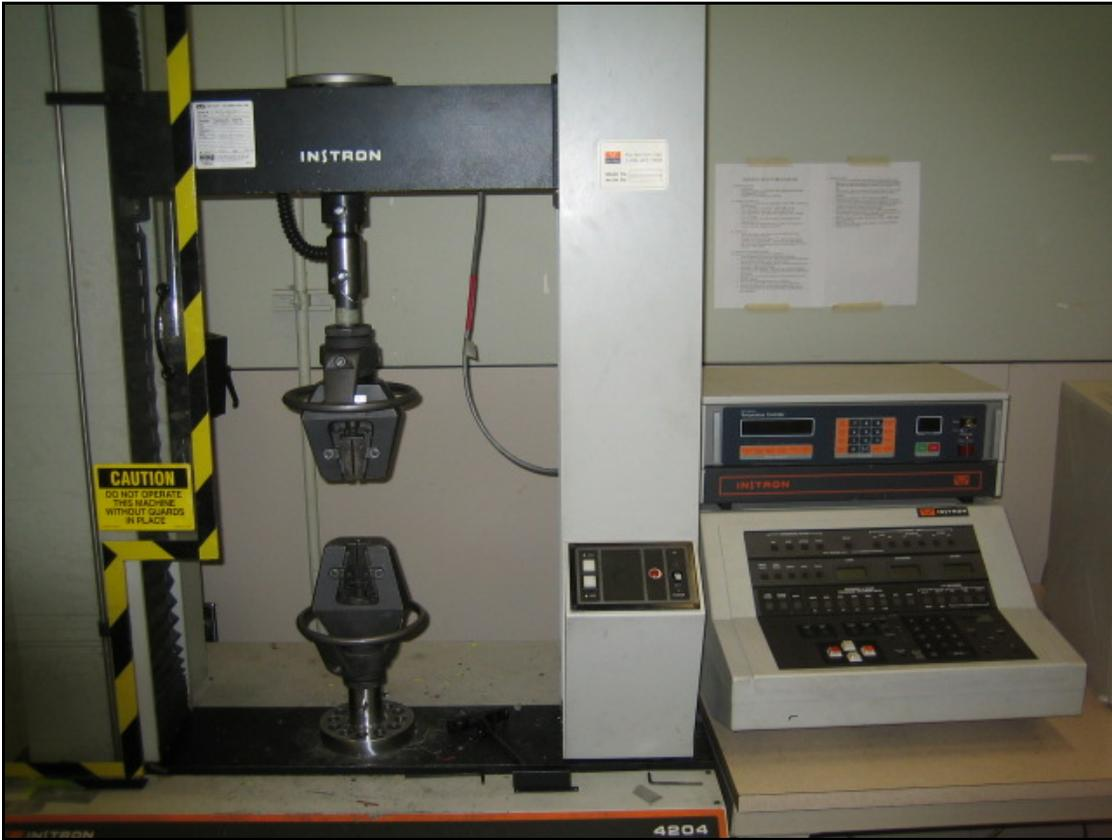
Figure 3-6 Instron tensile testing machine.
