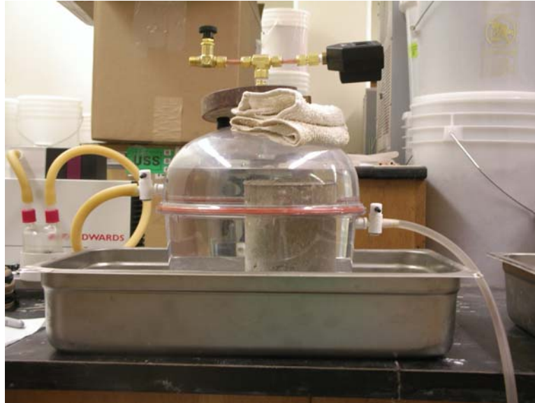
Figure 3.11 Vacuum saturation test configuration.
