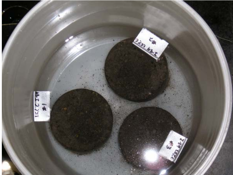
Figure 3.9 Soaking configuration for freeze-thaw testing.
