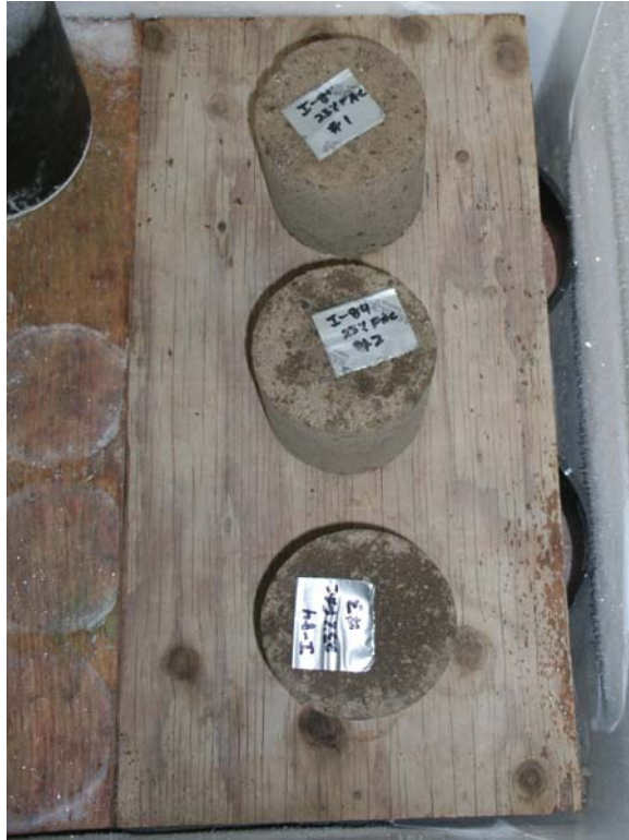
Figure 3.7 Freezing configuration for freeze-thaw testing.
