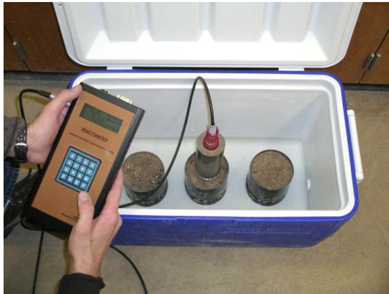
Figure 3.13 Tube suction test configuration.
