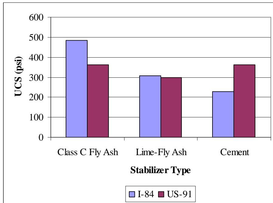
Figure 4.11 Interaction between aggregate type and stabilizer type for UCS after the freeze-thaw test.
