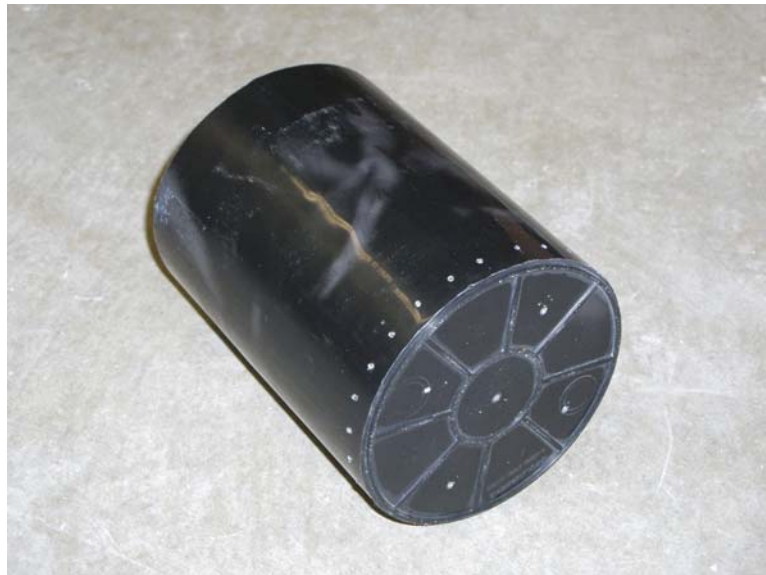
Figure 3.12 Plastic mold used for tube suction test.
