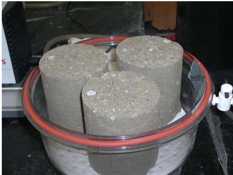
Figure 3.10 Vacuum chamber used for vacuum saturation test.
