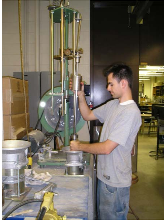
Figure 3.1 Compaction apparatus and finishing tool.
