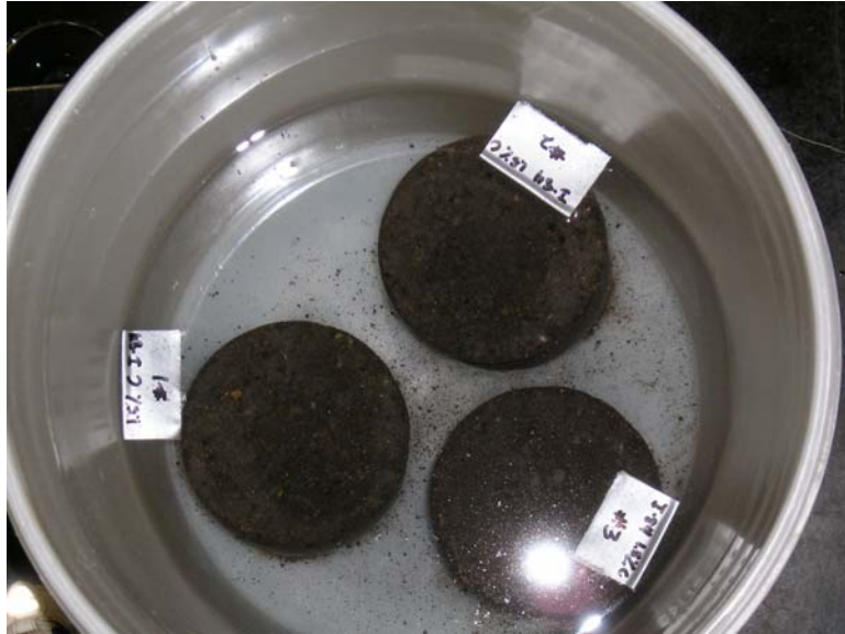
Figure 3.6 Specimens soaking prior to UCS testing.
