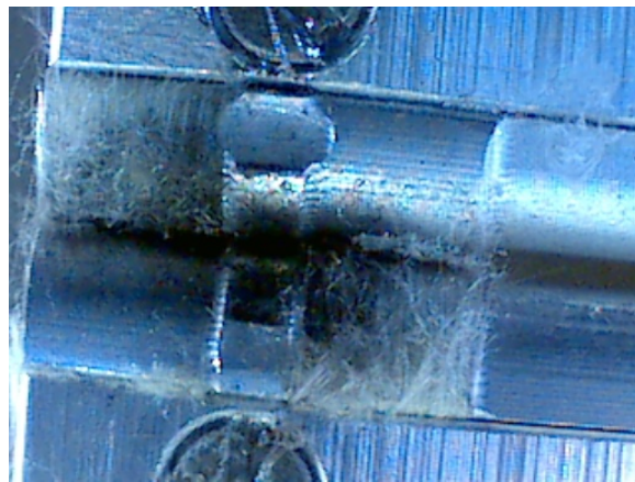
Figure 3.13: Abrasion of Kevlar fibers due to aluminum oxide
