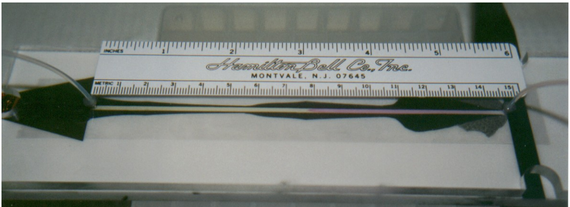
Figure III.13. Formation of a pH gradient in the separation channel. For conditions, see text.
