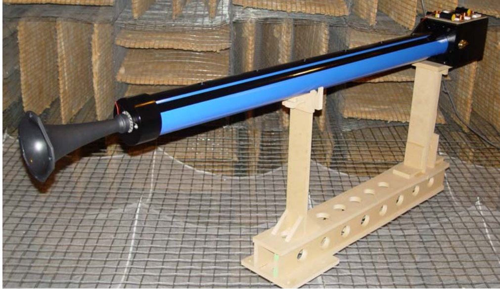
Figure 8.18. Long shotgun tube with high-frequency compression driver mounted on the end.
