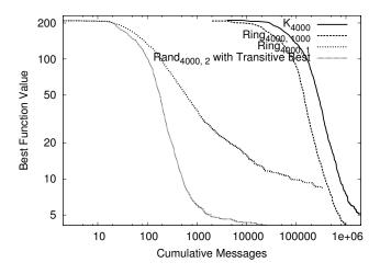
Fig. 16. PSO performance on Rastrigin with respect to communication.
