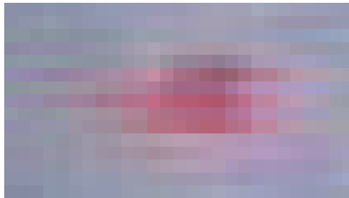
Figure 4.2: A close-up view of a red target as seen by a CCD camera (red darkened for grayscale contrast).
