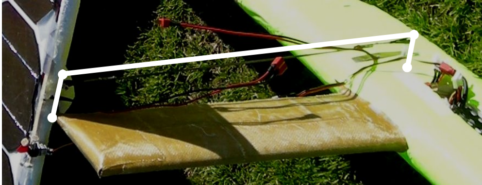
Fig. 3.5 The UAV laying on its side. The solar tracker four-bar linkage is highlighted in white. The servo body is housed in the fuselage, and the servo arm link is protruding out of the side of the fuselage.
