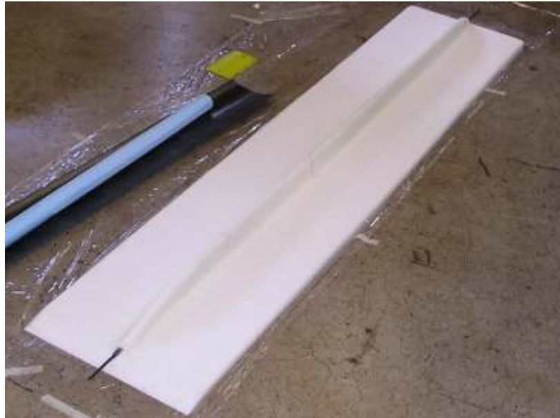
Fig. 4.4 Structural panel for the array of PV cells
