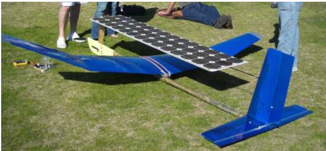
Fig. 2.2 The assembled NanSun. The tracker controller rotates the solar panel about the carbon rod that is attached to the tail's vertical stabilizer and the front tracker support panel.
