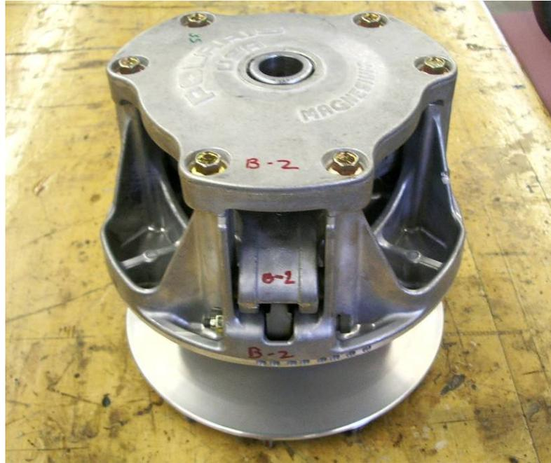
**Figure 3-4 Labeled primary clutch.**
