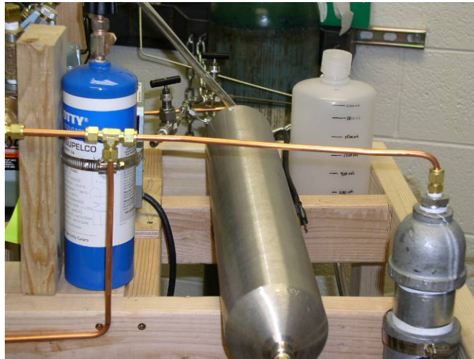
Figure 23. Ballast tank, V-101.
