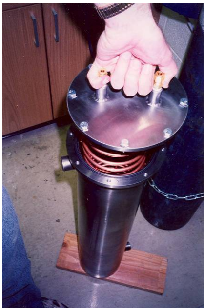
Figure 11. Heat exchanger used to cool liquid stream, E-102.
