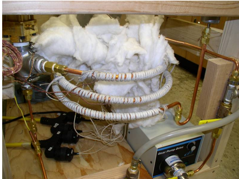
Figure 10. Heat exchanger used to heat liquid stream, E-101.
