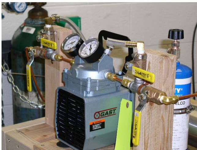
Figure 22. Vacuum/Pressure Pump, P-102.
