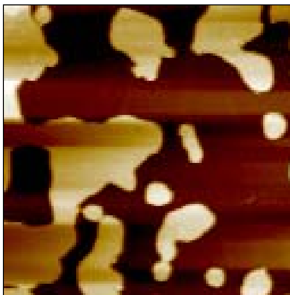
Fig. 2C. A few minutes after Fig. 2B. Image size: 3.0 \mu\text{m}^2 . Ht. scale: 0-8.5 nm. Notice destruction of lipid bridge at top.
