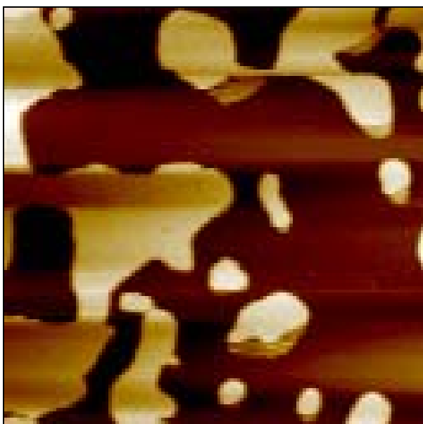
Fig. 2B. A few minutes after Fig. 2A. Image size: 3.0 \mu\text{m}^2 . Ht. scale: 0-8.7 nm. Notice absence of circular lipid patches.
