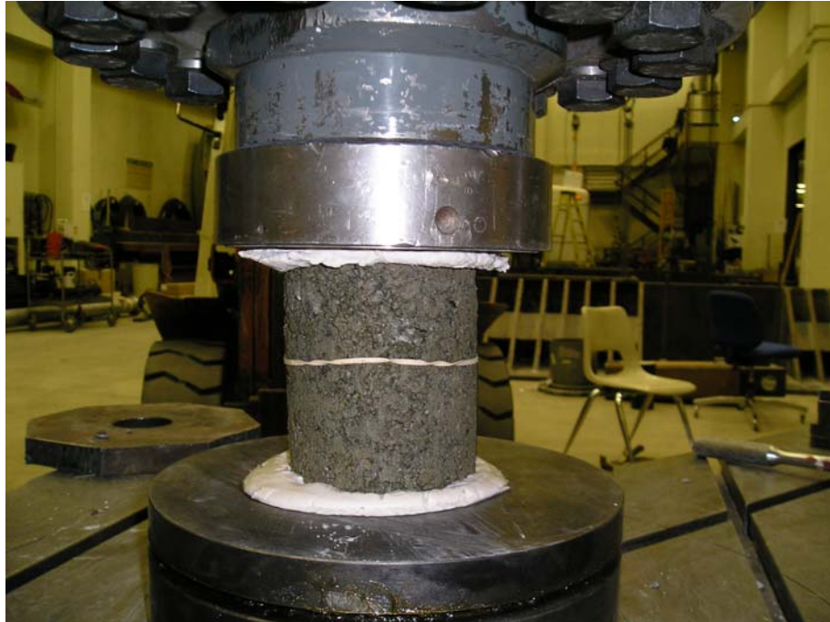
FIGURE 3.2 Test specimen subjected to UCS testing.
