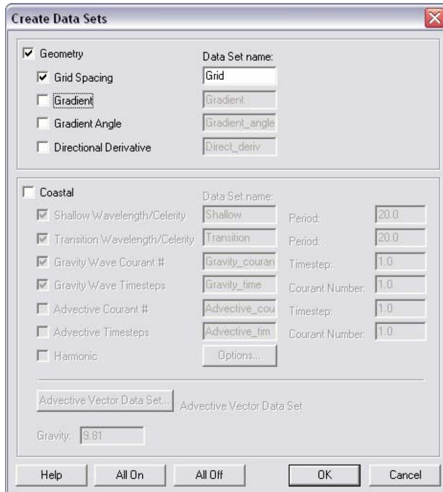
Figure 4.1-2 Create Data Sets Dialog in SMS used for Comparing LTEA Guidelines with Final Mesh Spacing
