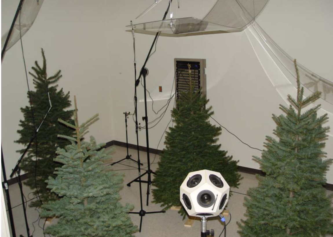
FIG. 7.2. Four Noble Fir trees and the dodecahedron loudspeaker in the reverberation chamber for sound absorption measurements during December 2004.
