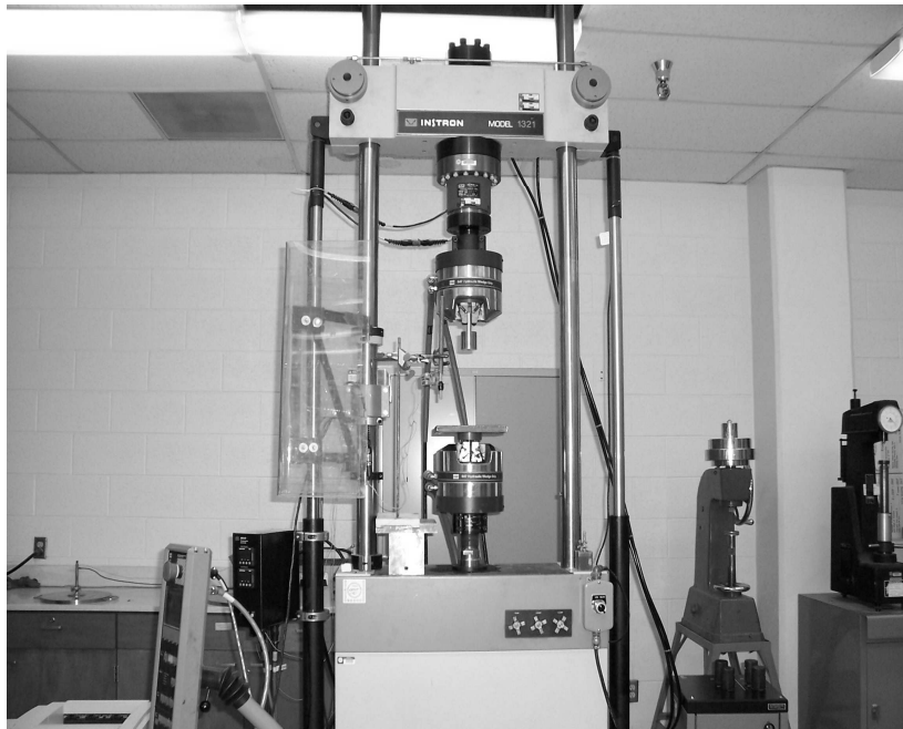
FIGURE 3.8 Loading frame used to conduct CBR testing.
