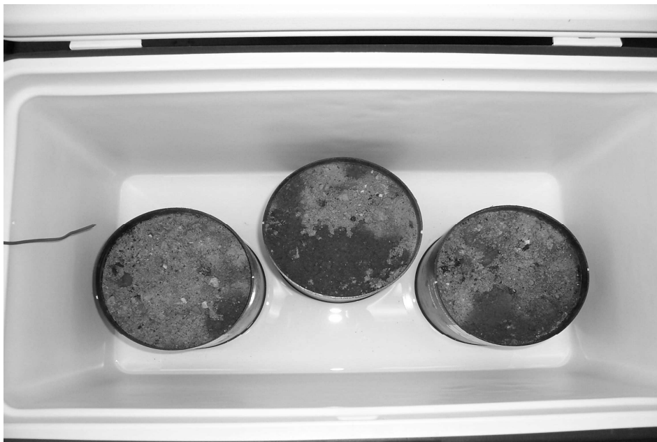
Figure 4.5 Water at surfaces of moisture-susceptible specimens.
