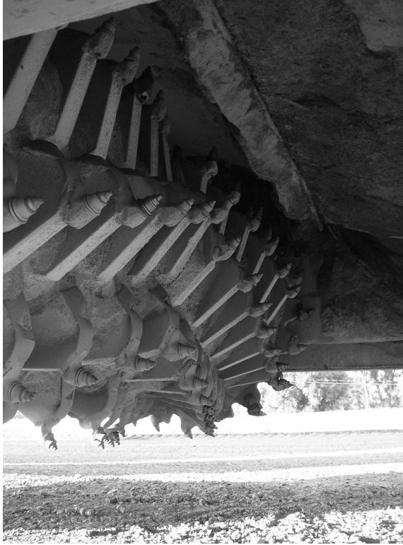
FIGURE 2.7 Metal teeth on rotating drum.
