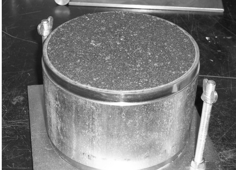
FIGURE 3.3 Compacted specimen in mold.
