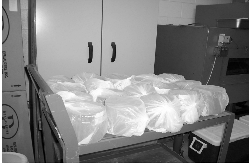
FIGURE 3.5 Specimens sealed in plastic bags prior to drying.
