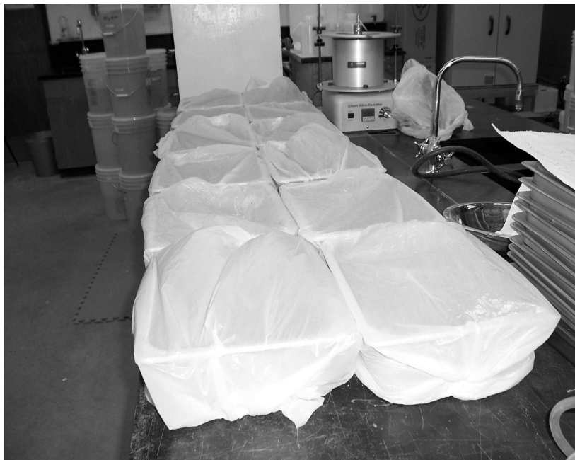
FIGURE 3.2 Soaking of aggregate samples.
