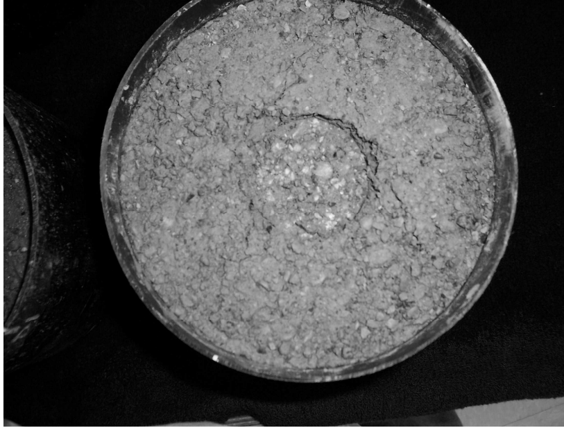
FIGURE 3.9 Typical surface indentation following CBR testing.
