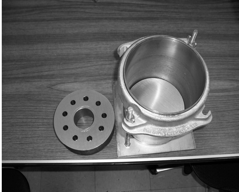
FIGURE 3.7 Metal mold used for CBR testing.
