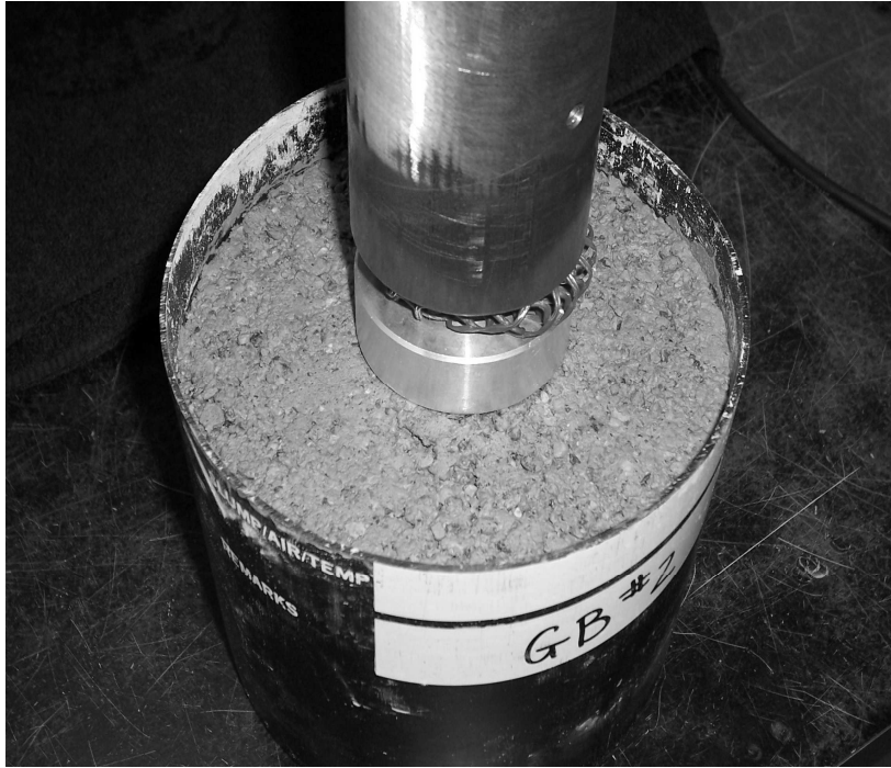
FIGURE 3.14 Probe used to measure dielectric and electrical conductivity values.
