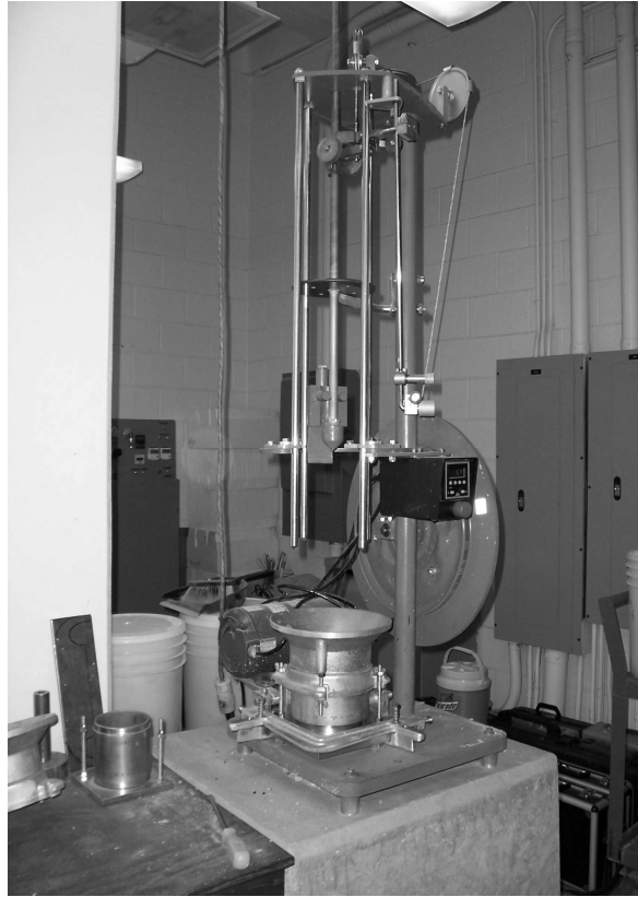
FIGURE 3.1 Mechanized compaction device.
