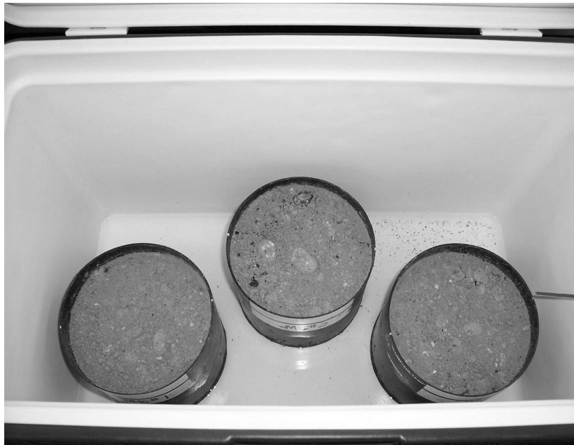
FIGURE 3.13 Capillary soaking in ice chest.
