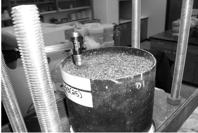
FIGURE 3.11 Striking the specimen surface with the instrumented hammer.
