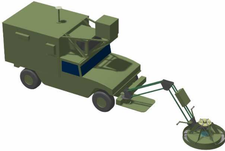
Figure 1.2: QM Landmine detection system. The primary sensor is mounted on a boom that extends from the front of the Humvee. The reference antennas are mounted on the top of the Humvee. Image courtesy Quantum Magnetics.
