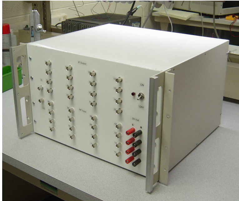
Figure 2.9: Box containing the receiver system.
