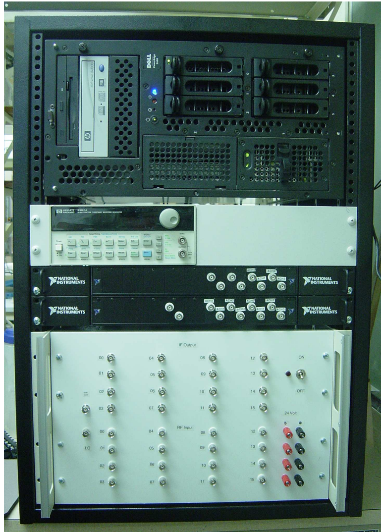
Figure 2.11: At the top of the rackmount is the computer in which the A/D cards are housed. Below that is a signal generator that provides the LO signal. Next are two breakout boxes and the receiver box. The outputs of the receiver box are connected to the A/D cards through the breakout boxes.
