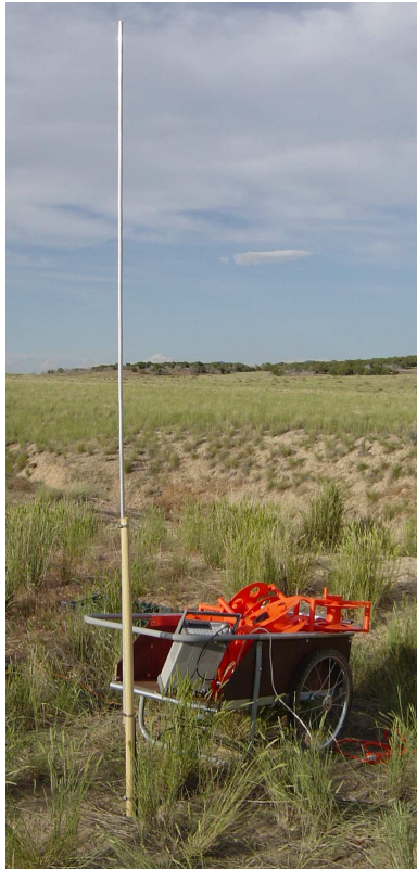
Figure 3.7: Picture of the calibration antenna. The signal generator can be seen just to the right of the antenna.
