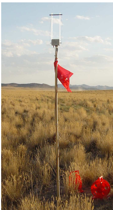
Figure 3.4: Picture of an antenna mounted on a wood mast. Red flags were attached to increase visibility of the antennas. The reels used to hold the power and signal cable can be seen at the mast base.
