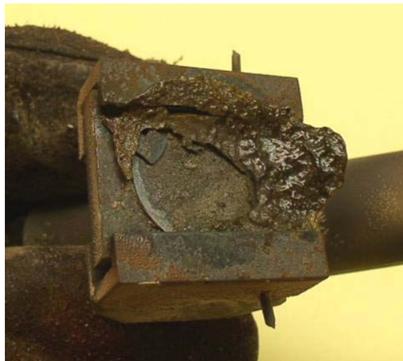
Figure 6. Photograph of accelerated deposits produced by a very high particulate loading.
