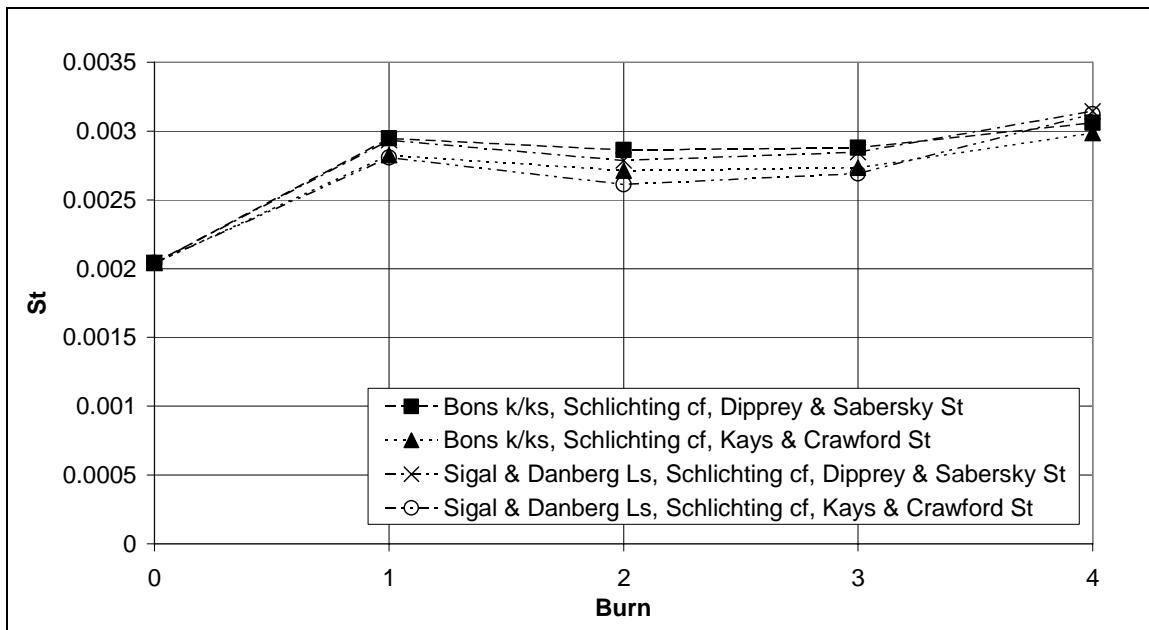
Figure 48. Stanton numbers derived from roughness correlations.
